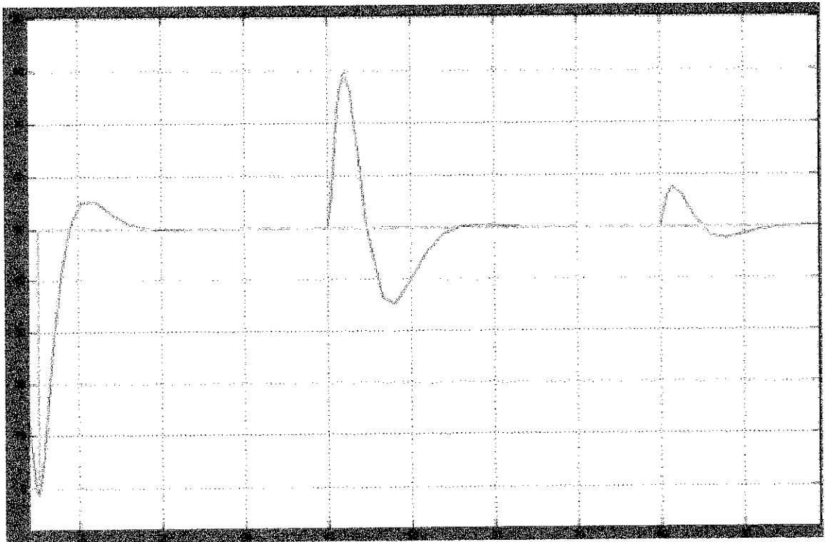
Figure 4.9: Cascade control loop with 2 disturbances
