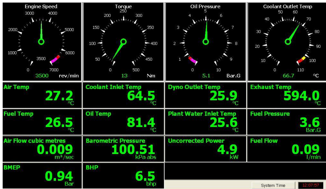
Figure 5.8: 3500 rev/min (without HOD System installed)
