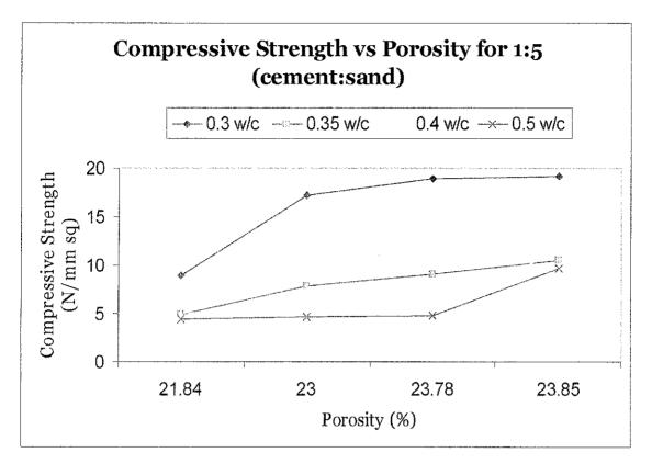
Figure 6.8: Compressive Strength vs Porosity for 1:5 (Cement: Sand) graph
