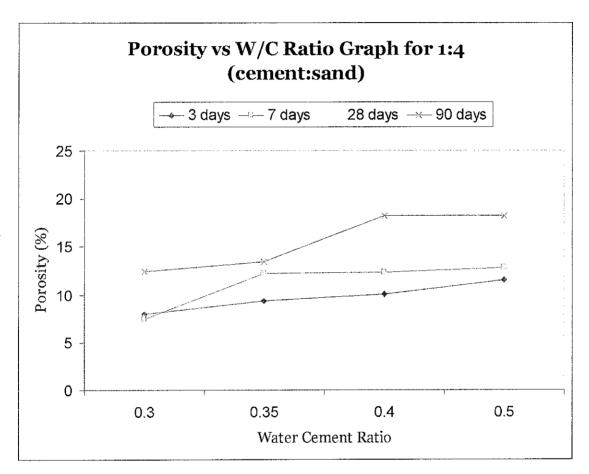
Figure 6.4: Porosity vs Water Cement ratio for 1:4 (Cement: Sand) graph
