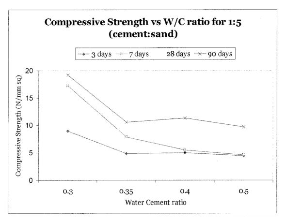
Figure 6.2: Compressive Strength vs Water Cement Ratio for 1:5 (Cement: Sand) graph
