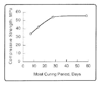
Figure 2.2: Relationship between compressive strength of mortar and moist curing age
