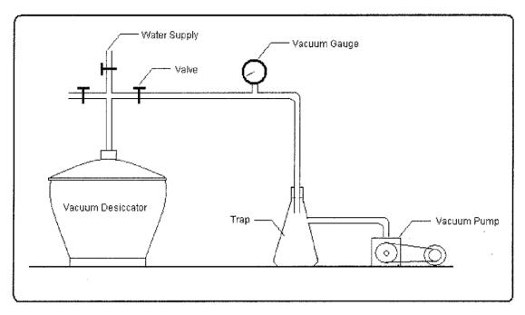
Figure 2.4: Vacuum Saturation Apparatus
