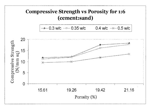
Figure 6.9: Compressive Strength vs Porosity for 1:6 (Cement: Sand) graph
