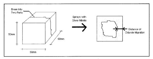
Figure 3.3: Chloride Migration Test
