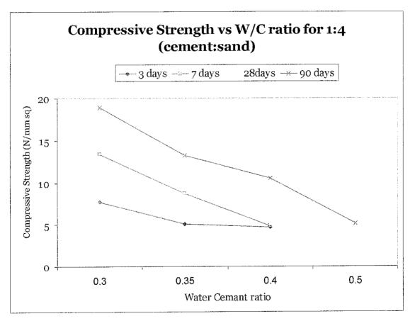
Figure 6.1: Compressive Strength vs Water Cement Ratio for 1:4 (Cement: Sand) graph
