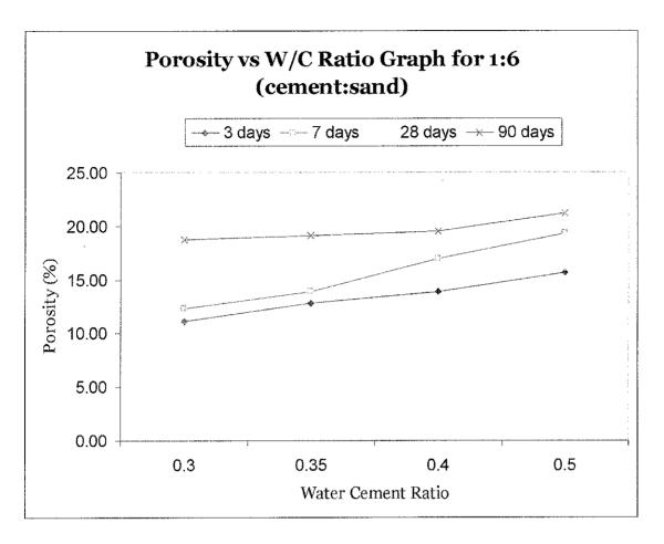
Figure 6.6: Porosity vs Water Cement ratio for 1:6 (Cement: Sand) graph
