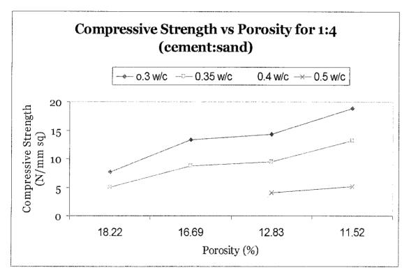
Figure 6.7: Compressive Strength vs Porosity for 1:4 (Cement: Sand) graph
