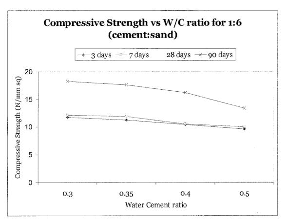
Figure 6.3: Compressive Strength vs Water Cement Ratio for 1:6 (Cement: Sand) graph
