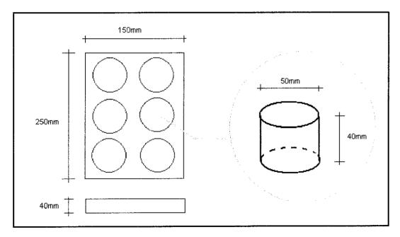
Figure 3.4: Dimension of Concrete Slab and Cored Concrete
