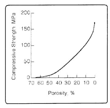
*Figure 2.3*: *The inverse relationship between porosity and strength of mortar*
