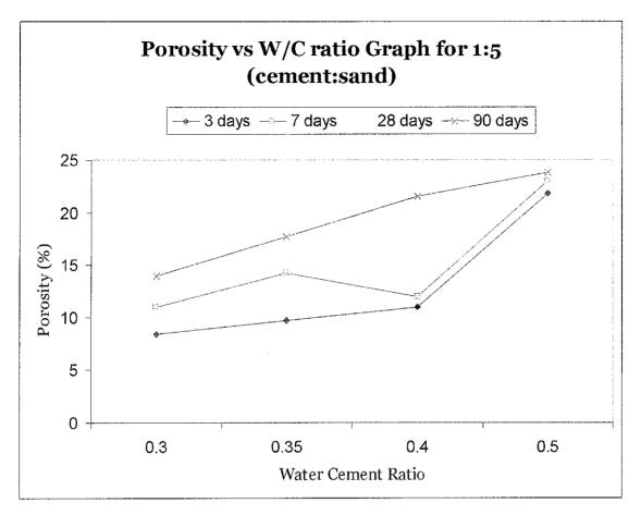
Figure 6.5: Porosity vs Water Cement ratio for 1:5 (Cement: Sand) graph
