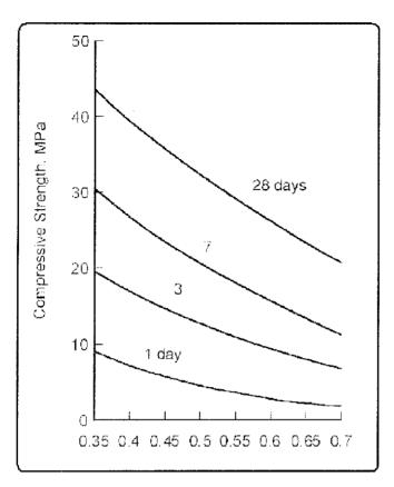
Figure 2.1: Influence of water cement ratio and moist curing age on mortar strength
