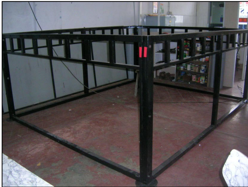
Figure 4.3 The Metal Structure of the House
