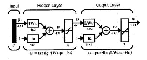
Basic Backpropagation network architecture is shown in figure 2.3. The number of hidden layers in a Feed Forward network is often one or more layers. Multiple layers of neurons with nonlinear transfer functions allow the network to adapt and learn nonlinear
