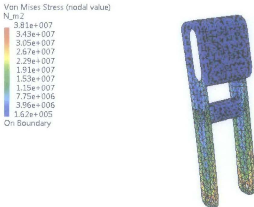
Figure 4.8: Redesigned brake pedal after FEA analysis showing the reduction in global maximum stress
