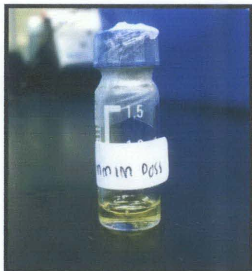
Figure 14 : 1-methyl-3-propionitrile imidazolium DOSS
