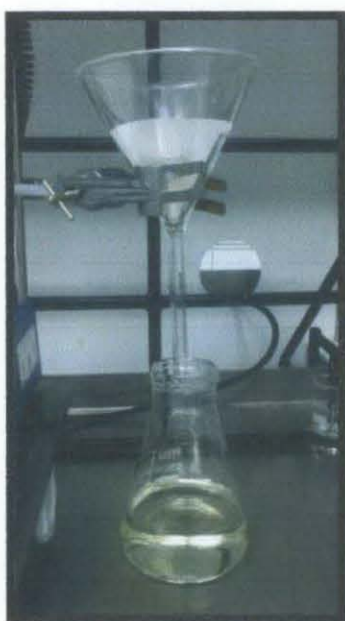
Figure 13 : Filtering remaining NaCl
