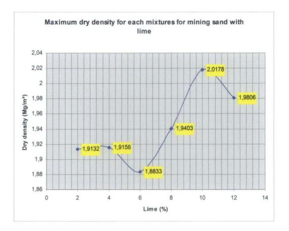
Figure 4.2: Percentage lime versus maximum dry density for the various percentage of lime used in each of the sample mixtures.
