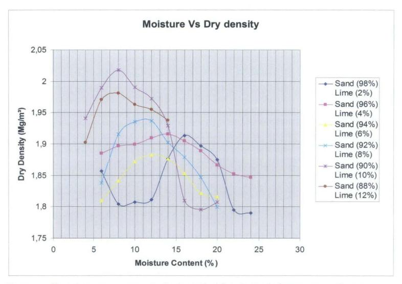
Figure : The moisture content versus dry density obtained from the standard proctor compaction test.
