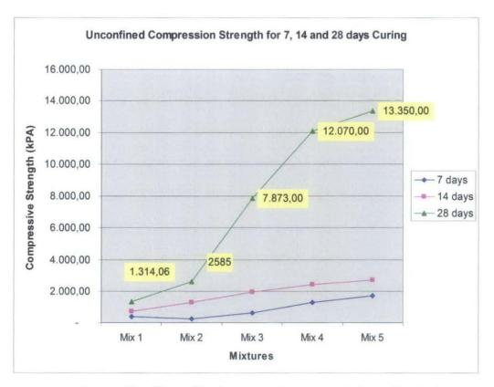
Figure 4.9: Unconfined compression strength for each of mixtures based on percentage of PFA and curing for 7, 14 and 28 days.
