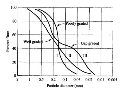
Figure 2.2: Different type of particle-size distribution curves. (Das 2002)
