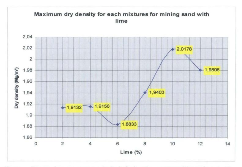
**Figure:** Percentage lime versus maximum dry density for the various percentage of lime used in each of the sample mixtures.
