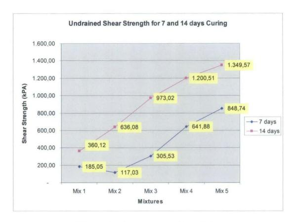
Figure 4.10: Undrained Shear Strength for each of mixtures based on percentage of PFA and 7 and 14 days curing period
