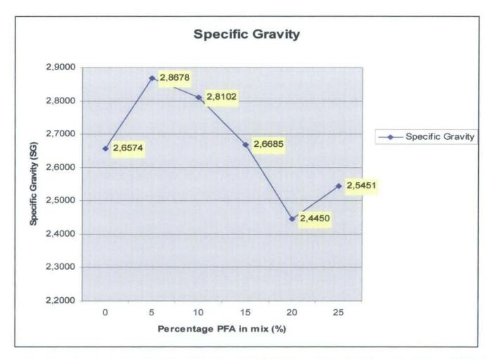
Figure : Specific gravity for mixtures of mining sand with PFA and lime based on percentage of PFA in each mix.
