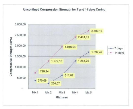
Figure 4.8: Unconfined compression strength for mixtures based on percentage of PFA and curing for 7 and 14 days.
