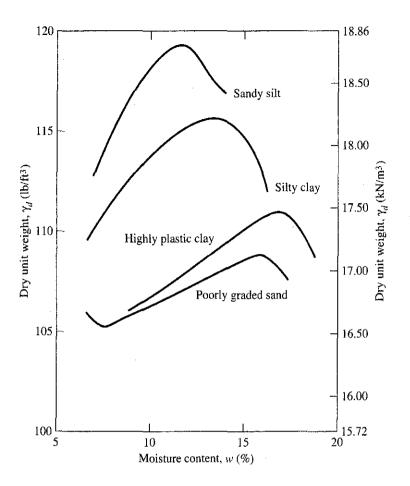
Figure 2.3: Typical compaction curves for four soils. (ASTM D-698)
