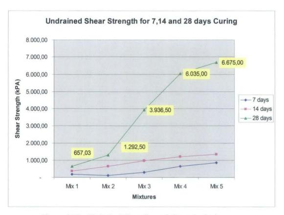
Figure 4.11: Undrained Shear Strength for each of mixtures based on percentage of PFA and 7, 14 and 28 days curing period.
