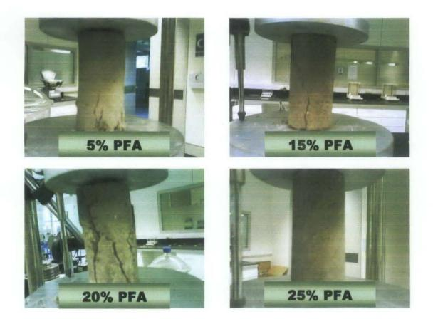
Figure: Unconfined Compression Test for 7 days Curing Period.
