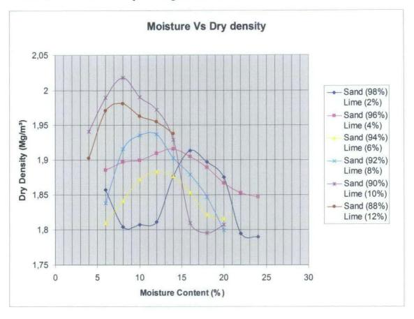
Figure 4.1: Moisture content versus maximum dry density from standard proctor compaction for mining sand mix with various percentage of lime.
