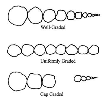
Figure 2.1: Three types of gradation from sieve analysis. They are well-graded, uniformly graded and gap graded soil.
