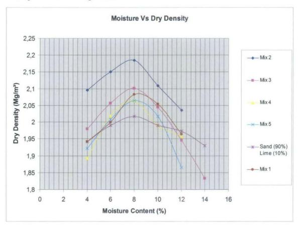
Figure 4.6: The moisture content versus dry density obtained from the standard proctor compaction test.
