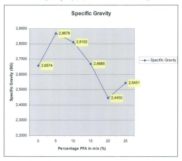
Figure 4.5: Specific gravity for mixtures of mining sand with PFA and lime based on percentage of PFA in each mix.
