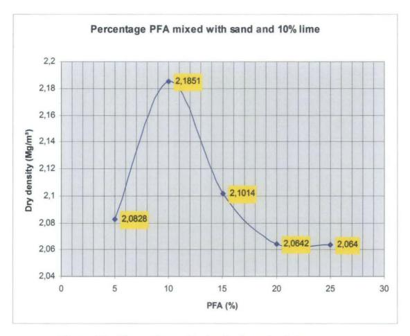
Figure 4.7: The maximum dry density for each mixture.
