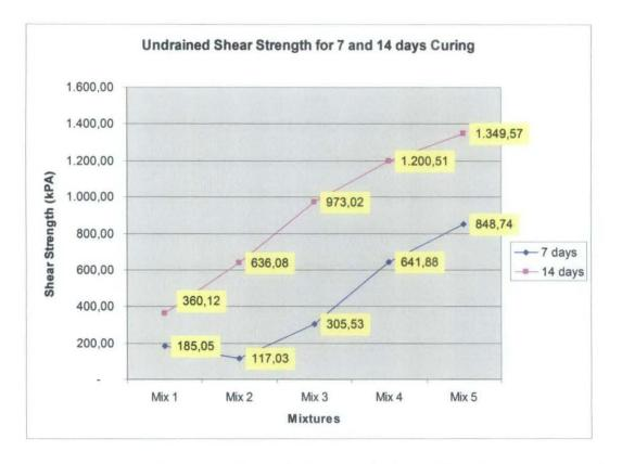
Figure: Undrained Shear Strength for each of mixtures based on percentage of PFA and 7 and 14 days curing period.
