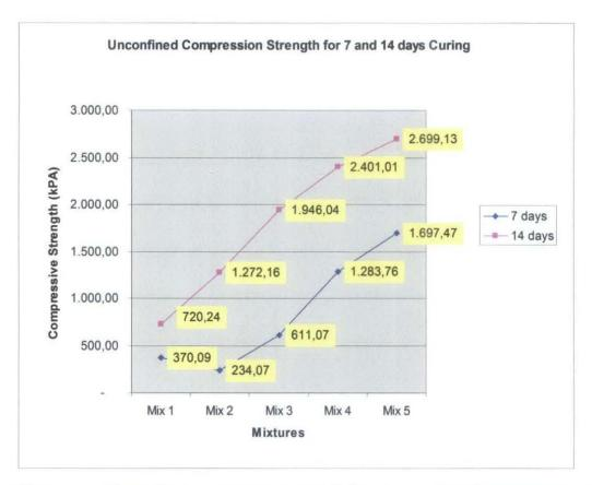
Figure: Unconfined compression strength for mixtures based on percentage of PFA and curing for 7 and 14 days.
