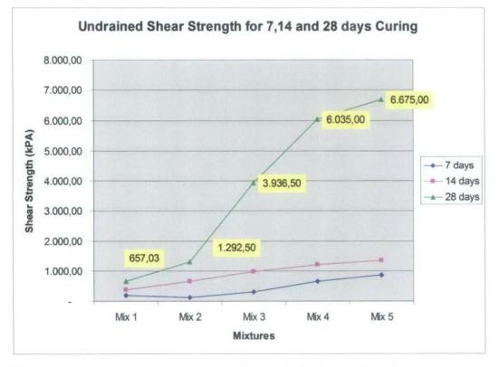
Figure: Undrained Shear Strength for each of mixtures based on percentage of PFA and 7, 14 and 28 days curing period.
