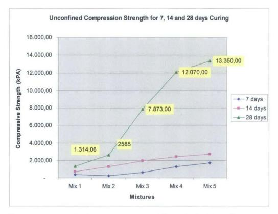
Figure: Unconfined compression strength for each of mixtures based on percentage of PFA and curing for 7, 14 and 28 days.
