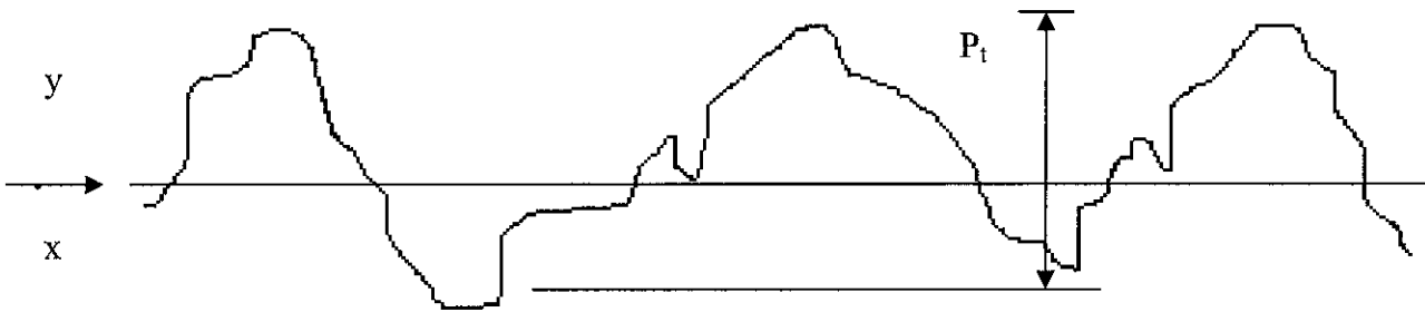
Figure 2.3 Sketch of a surface roughness profile
