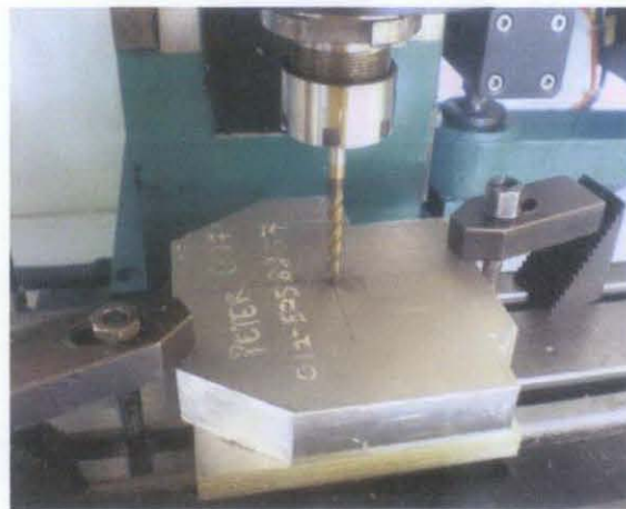
Figure 33: The hollow part of the palm is cut out
