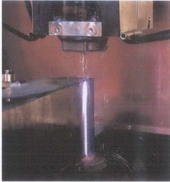
Figure 34: Wire EDM is cutting a metal block
