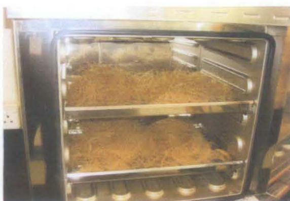
Figure 3.3: Oil Palm Fibres heated in Oven at 70°C for 24 hours
