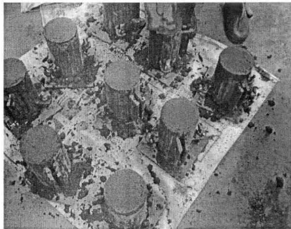
Figure 3.2: Casting of cylinder concrete
