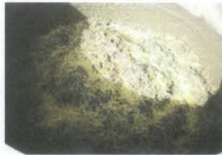
Mixing PVA fibers in the mix
