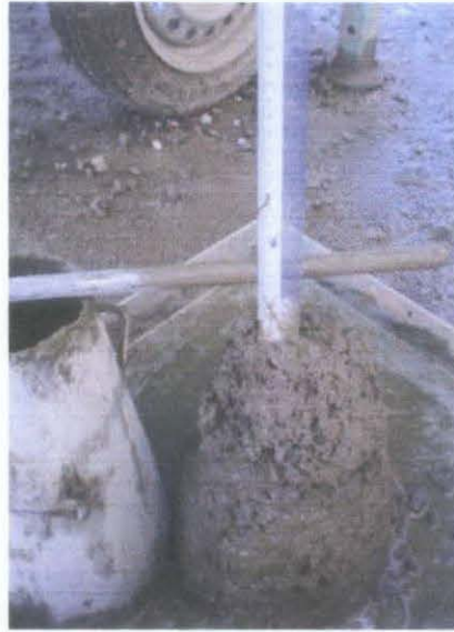
Figure 3.2: Slump test done for 2% PVA volume
