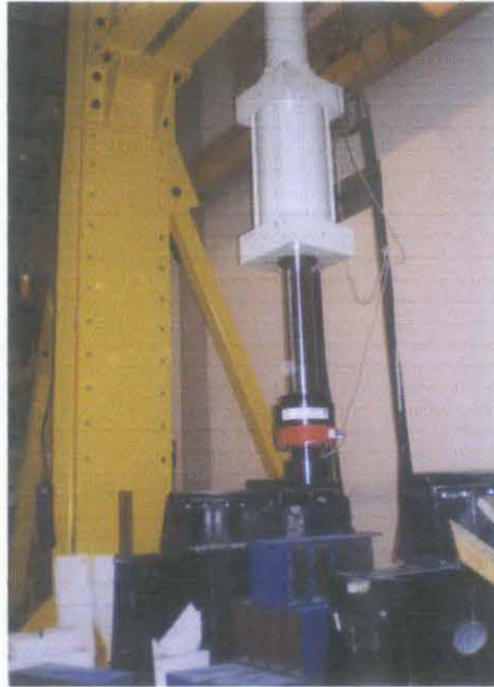
Figure 3.4: Dynamic compression test using UTM
