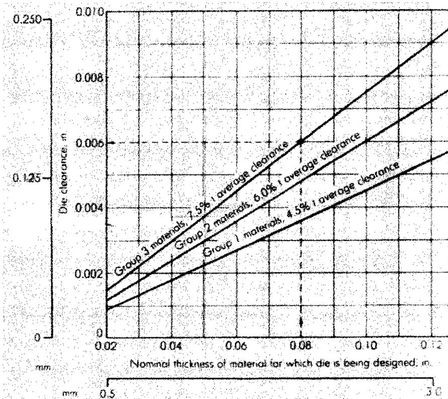
Figure 4.6 Die Clearances for Different Groups of Metals [3]
