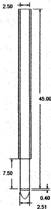
**Figure 4.9 The Designed Pilot**
