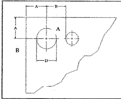
**Figure 4.11 Minimum Proportions for the Spacing of Holes from Corners of Die Block [1]**
