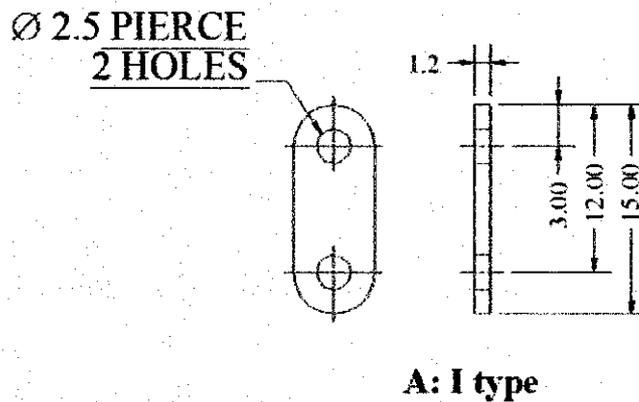
**Figure 4.3 Dimensions of the Metal Implant**
