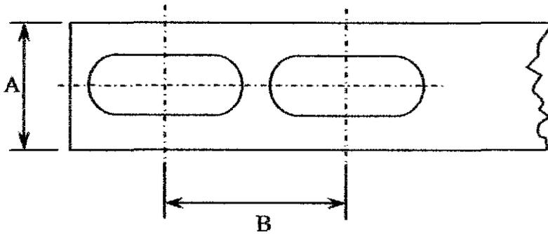
$$\begin{aligned} \text{Blank Area} &= A \times B \\ &= 10 \text{ mm} \times 15.84 \text{ mm} \\ &= \underline{\underline{158.4 \text{ mm}^2}} \end{aligned}$$
