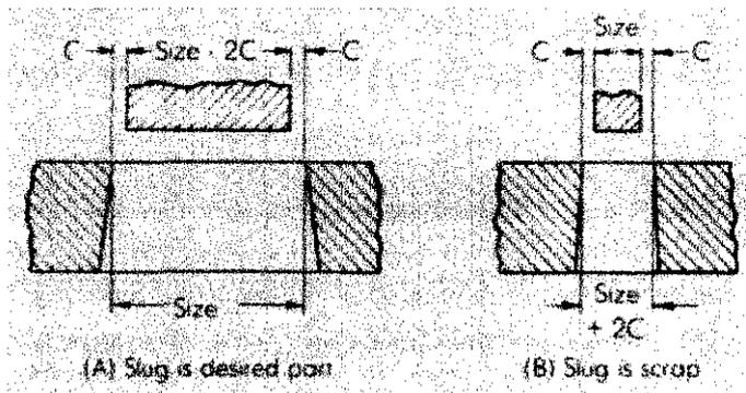
Figure 2.8 Control of Hole and Blank Sizes by Clearance Location [3]
