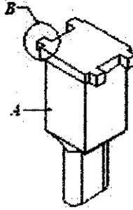
Figure 4.7 Design of the Blanking Punch [5]
