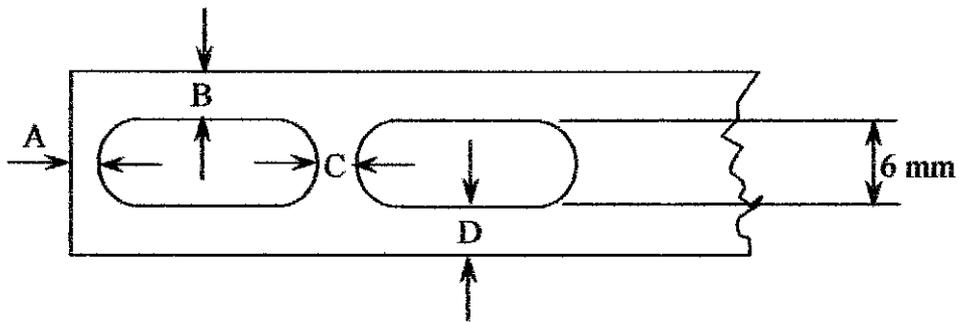
$$A = C = \frac{70}{100} \times T = \frac{70}{100} \times 1.2 \text{ mm} = \underline{\underline{0.84 \text{ mm}}}$$
