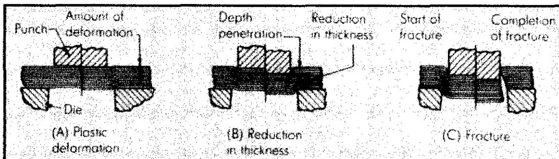
**Figure 2.2 Steps in Shearing Metal [3]**
