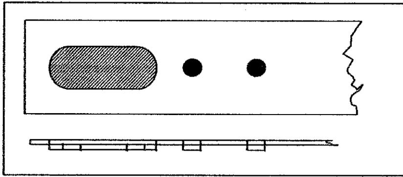
Figure 4.4 Blank Layouts Necessitating Narrow Strips
