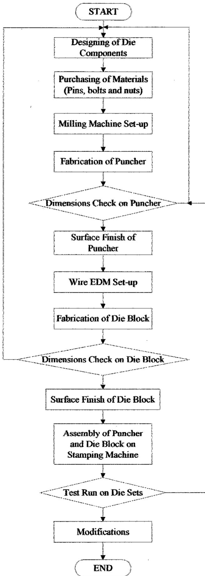
**Figure 3.3 Steps in Fabrication of Die Components**
