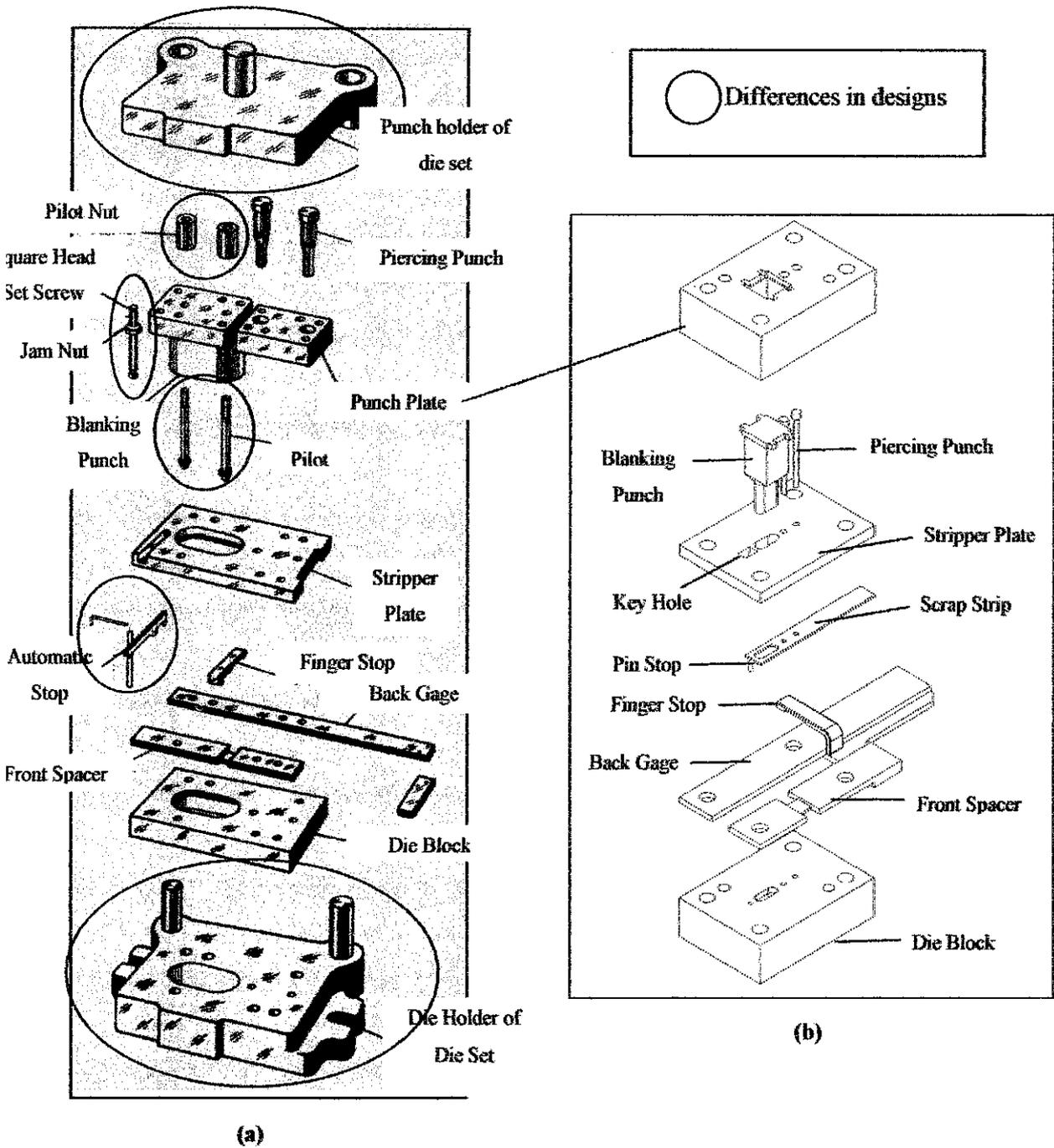
Figure 4.1 Exploded View of Die Components (a) Extracted from Reference Book [1]
