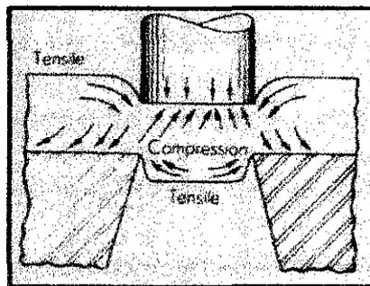
Figure 2.1 Stresses in Die Cutting [3]
