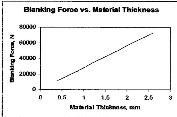
Figure 4.5 Relationship between Blanking Force and Material Thickness
