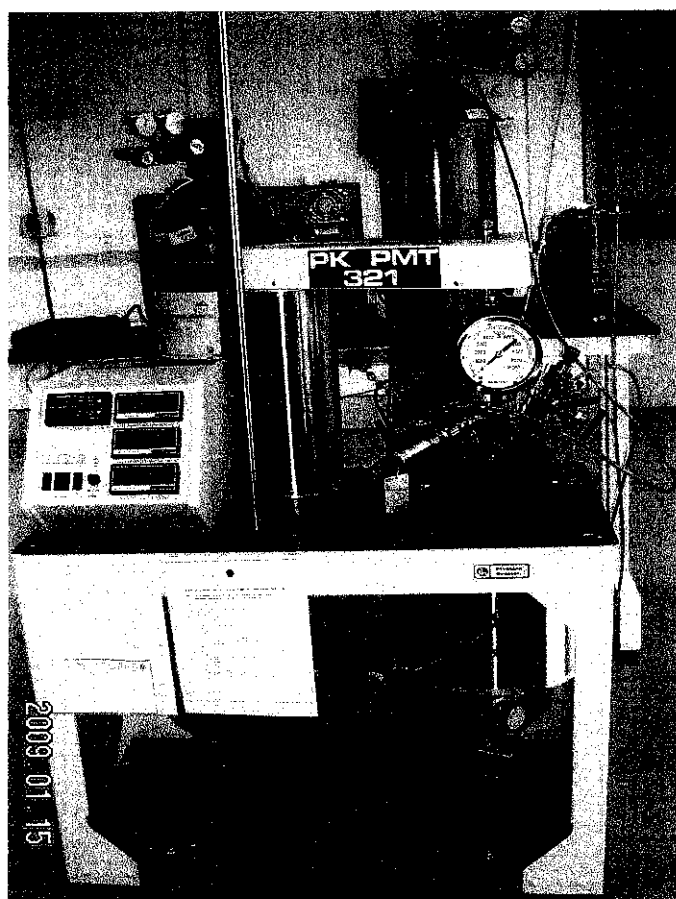
Figure 4.5: Parr high pressure reactor
