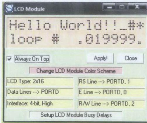
Figure 11: Simulation of LCD Display using PIC Simulator
