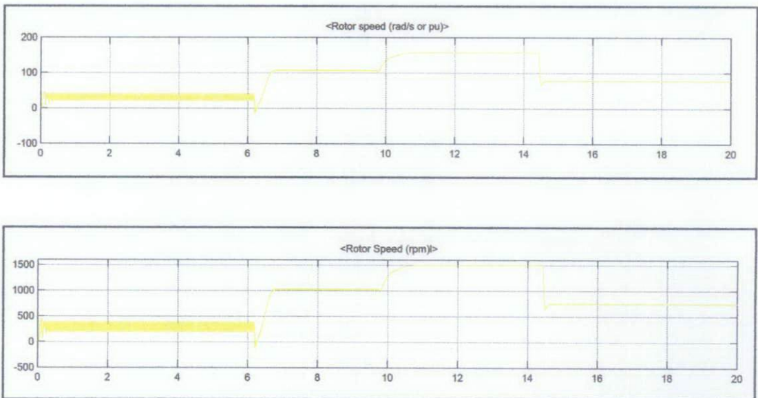
Figure 19 : The motor characteristic when varying the speed
