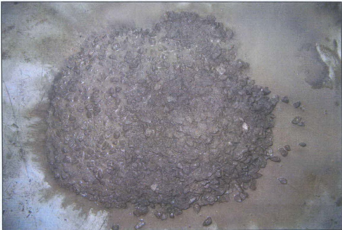
Figure E.2 Slump flow inner diameter 475 mm of size range 10mm – 14 mm
