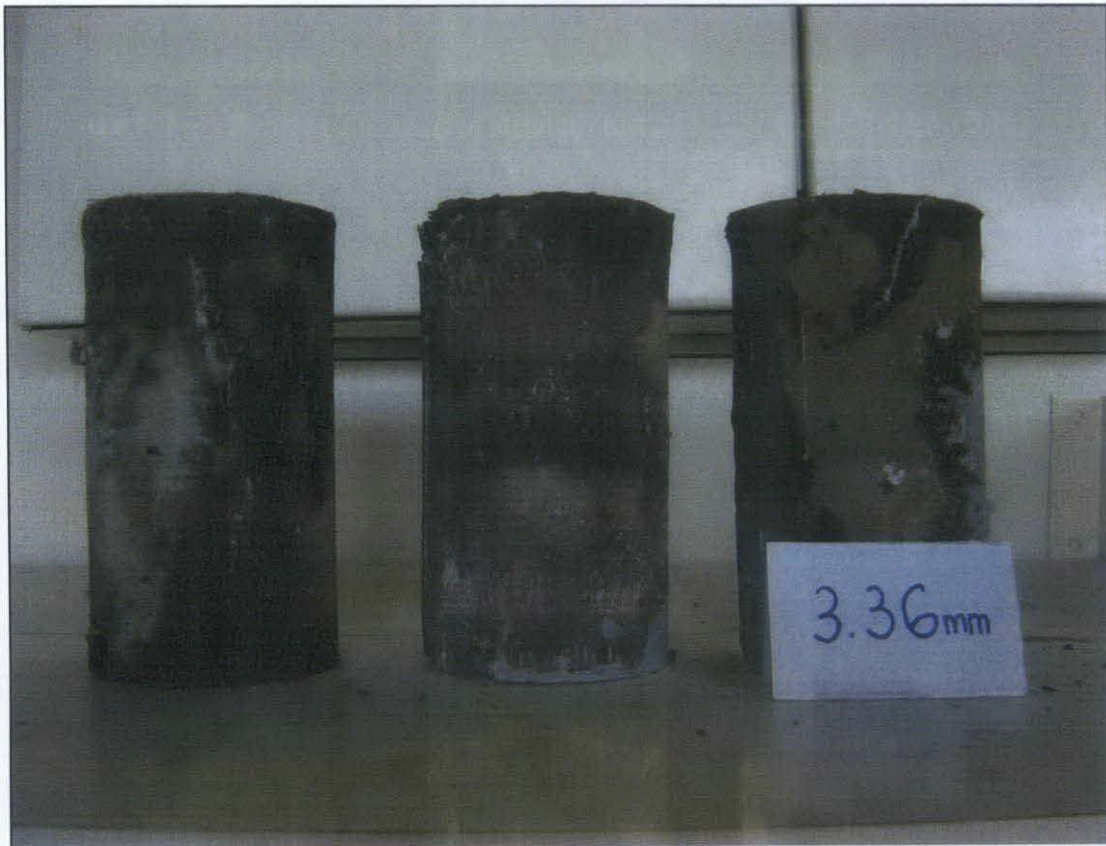
Figure F.8 After compressive strength test of size range 3.36 mm - 5 mm
