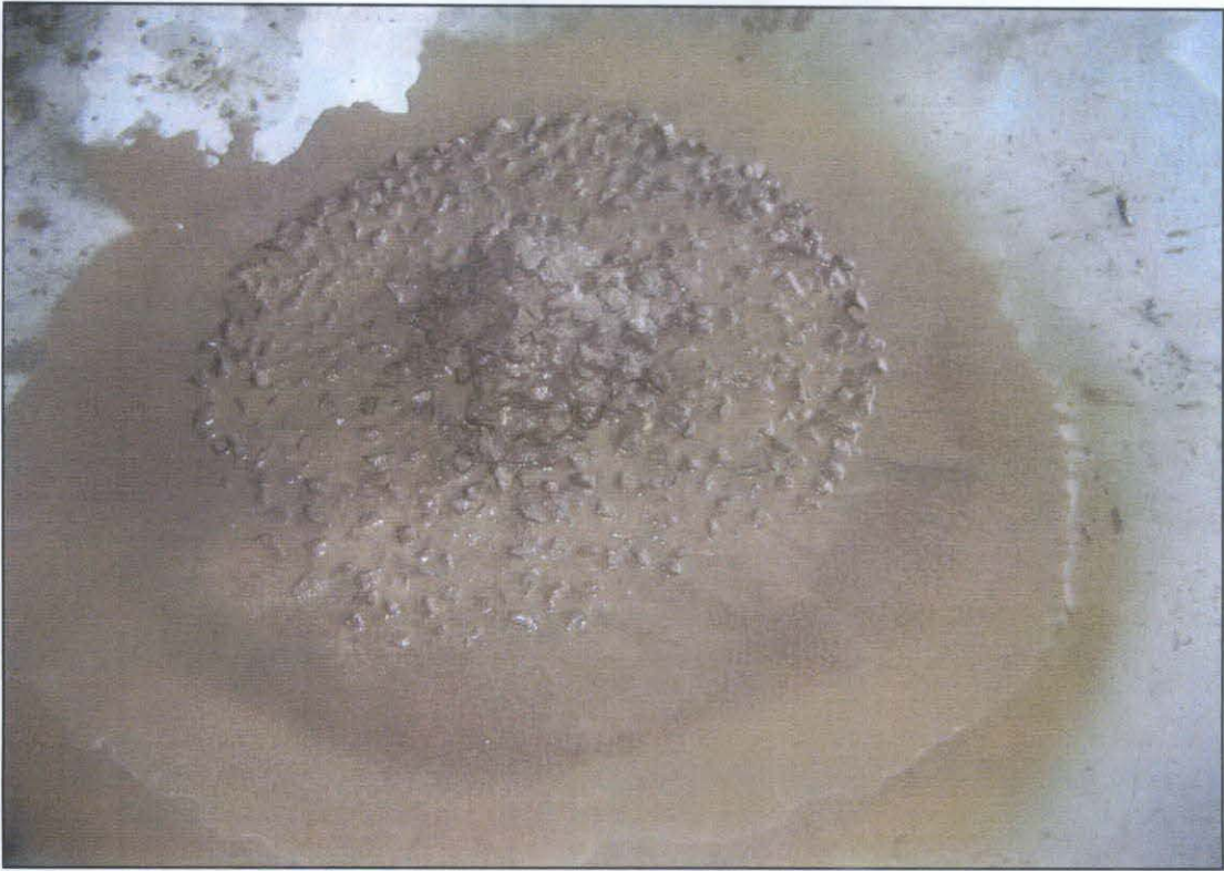
Figure E.1 Slump flow inner diameter 525 mm of size range 14mm – 20 mm
