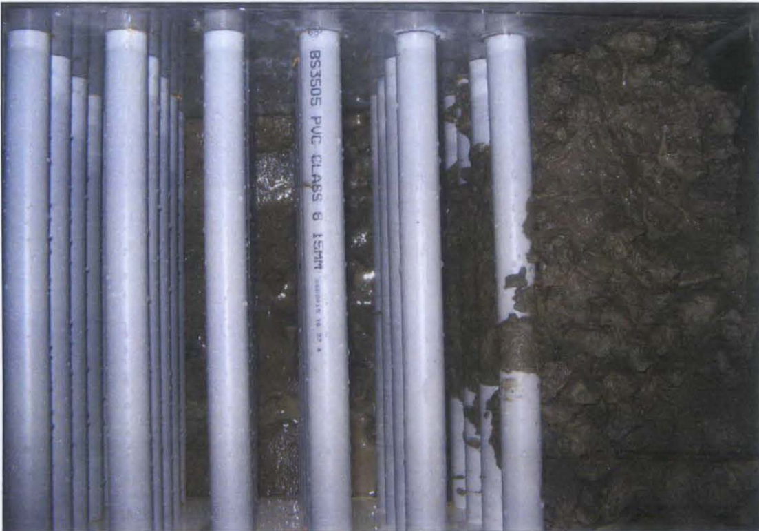
Figure D.2 Top view in Kajima Box of size range 14 mm – 20 mm
