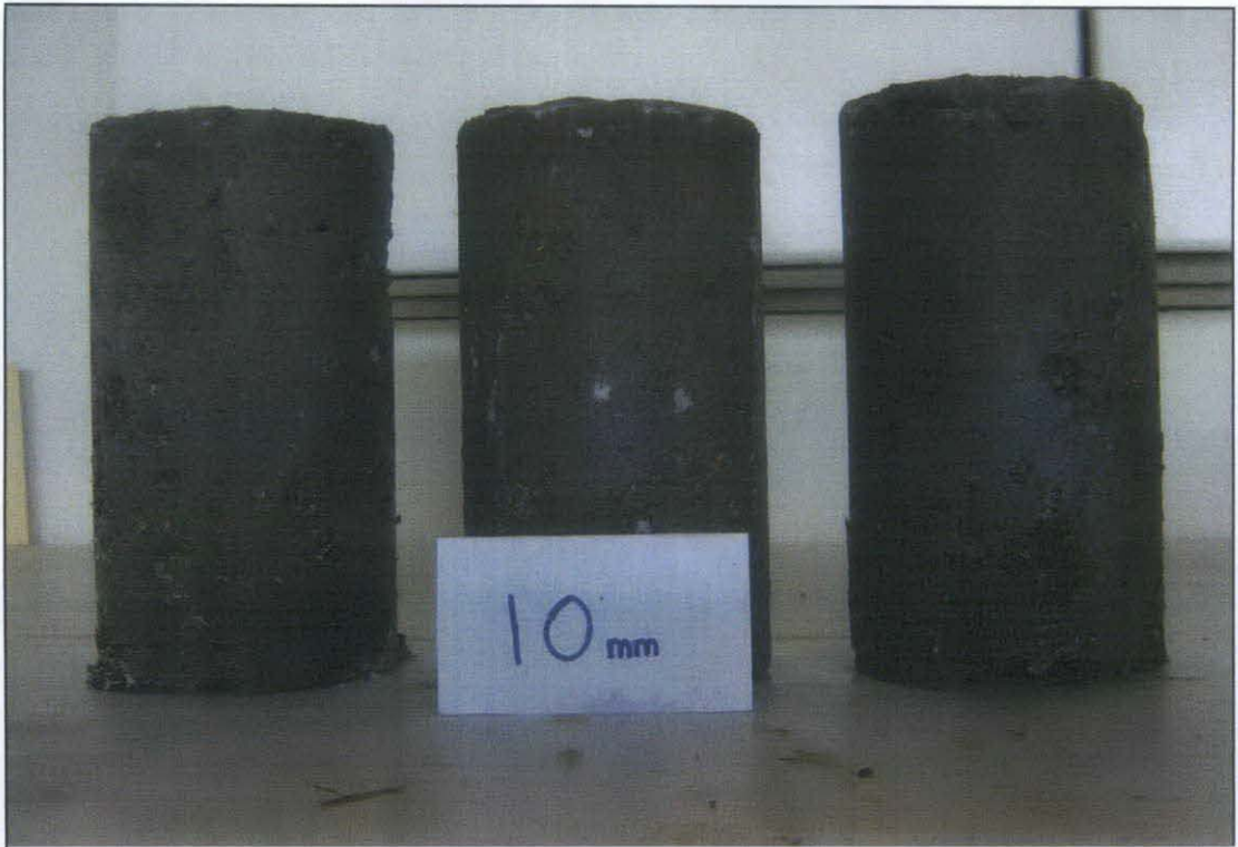
Figure F.3 Before compressive strength test of size range 10 mm - 14 mm
