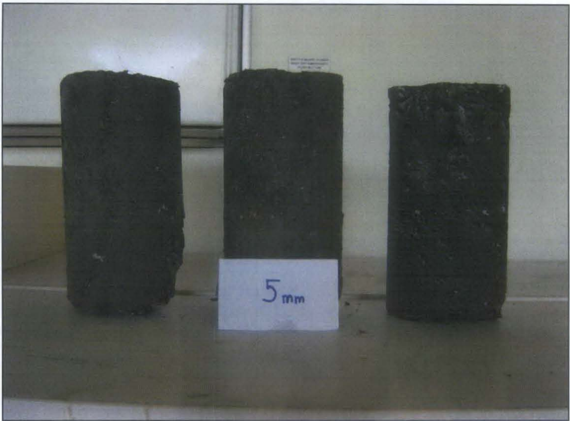
Figure F.5 Before compressive strength test of size range 5 mm - 10 mm
