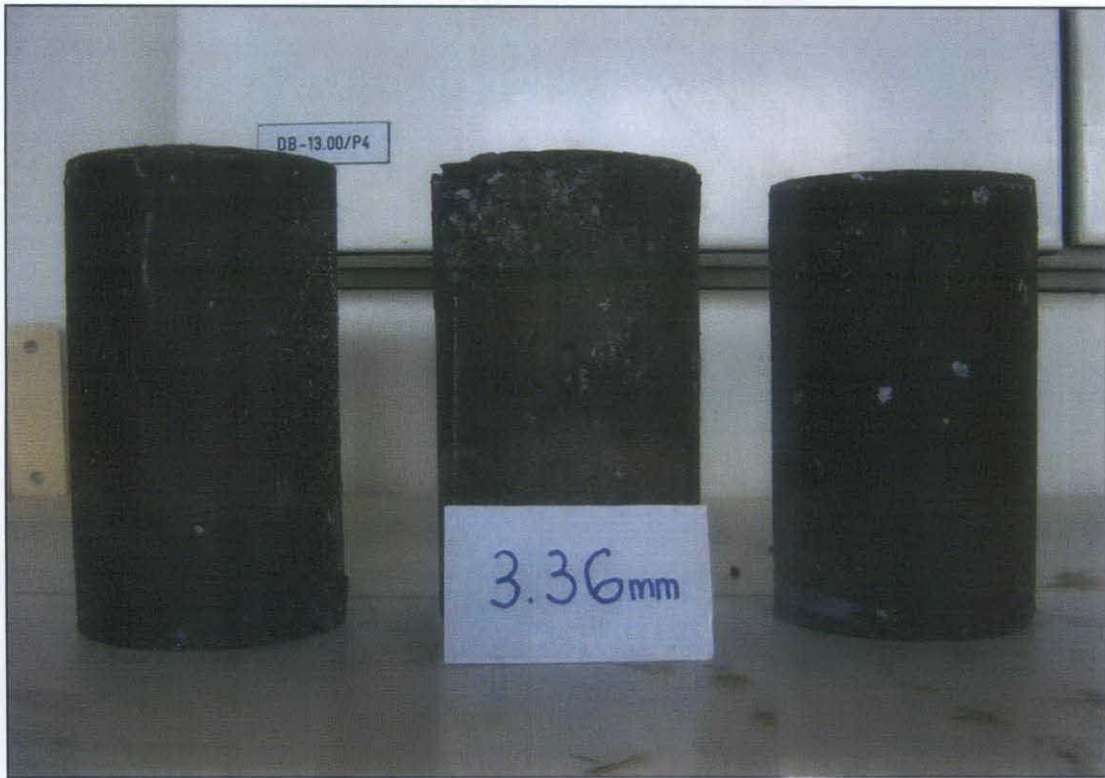
Figure F.7 Before compressive strength test of size range 3.36 mm - 5 mm
