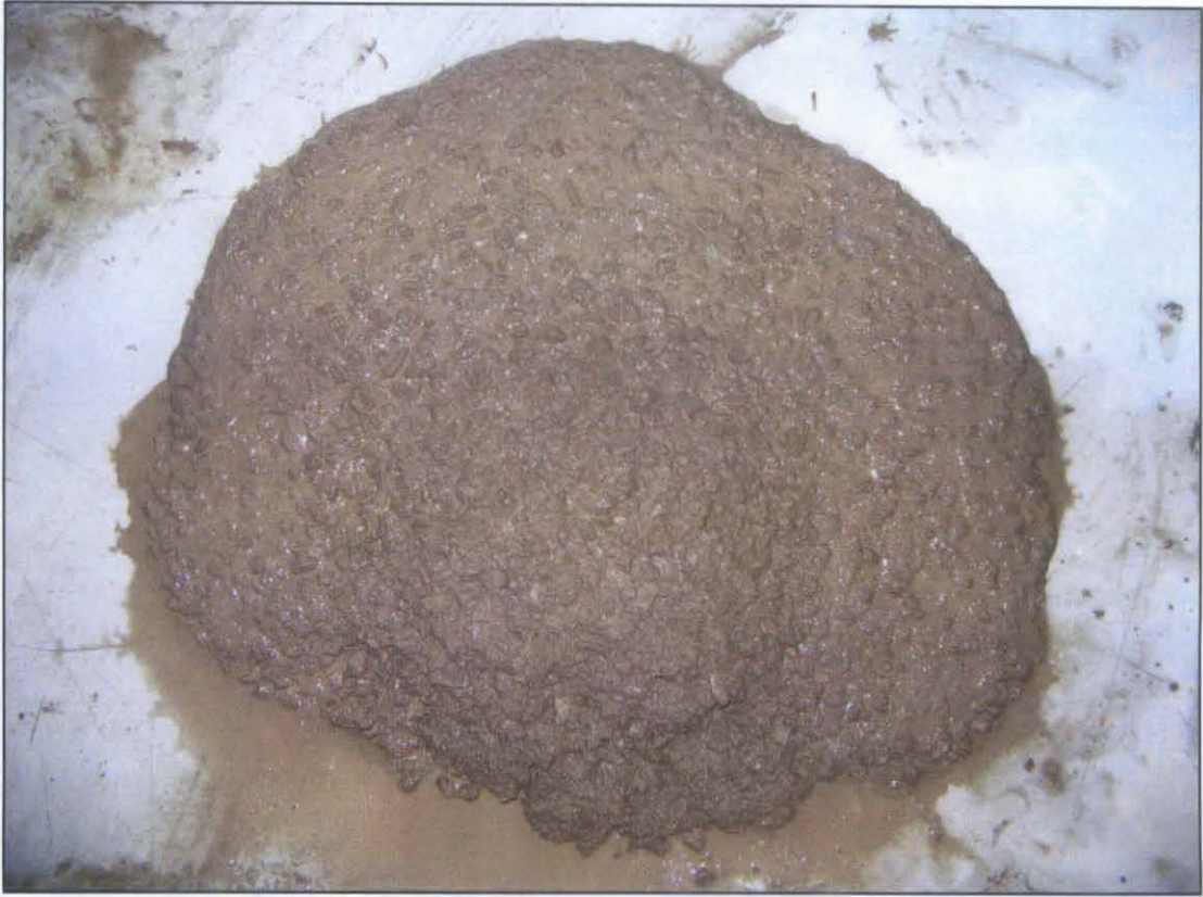
Figure E.3 Slump flow inner diameter 460 mm of size range 5mm – 10 mm
