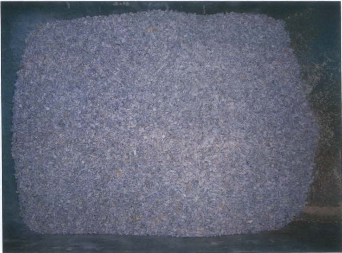
Figure I.4 Coarse aggregate of size range 3.36 mm – 5 mm
