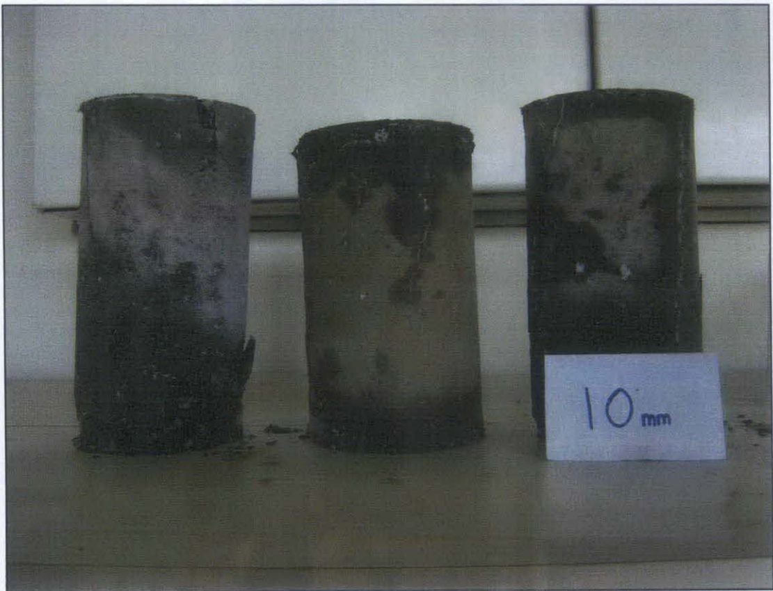
Figure F.4 After compressive strength test of size range 10 mm - 14 mm
