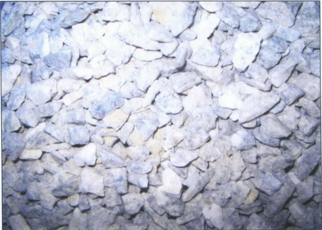
Figure I.2 Coarse aggregate of size range 10 mm - 14 mm
