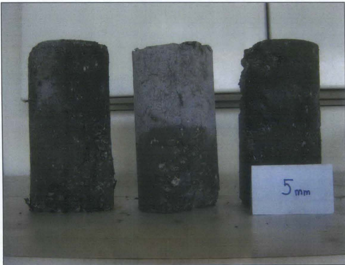
Figure F.6 After compressive strength test of size range 5 mm - 10 mm
