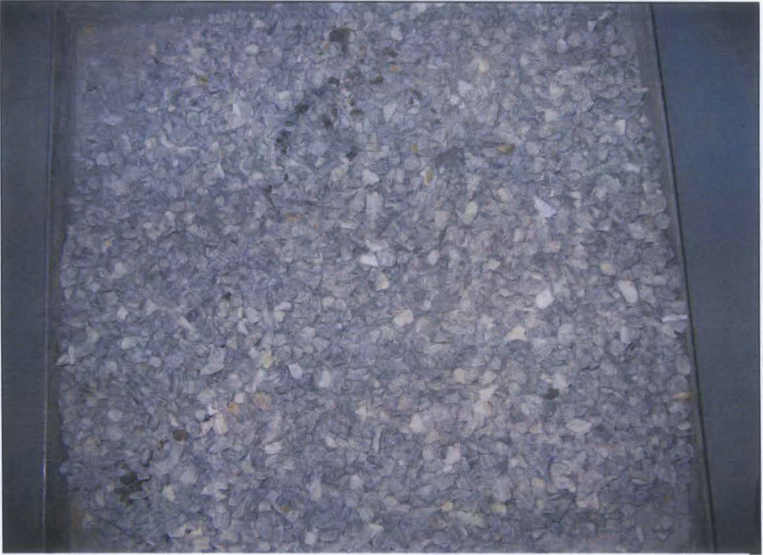
Figure I.3 Coarse aggregate of size range 5 mm - 10 mm
