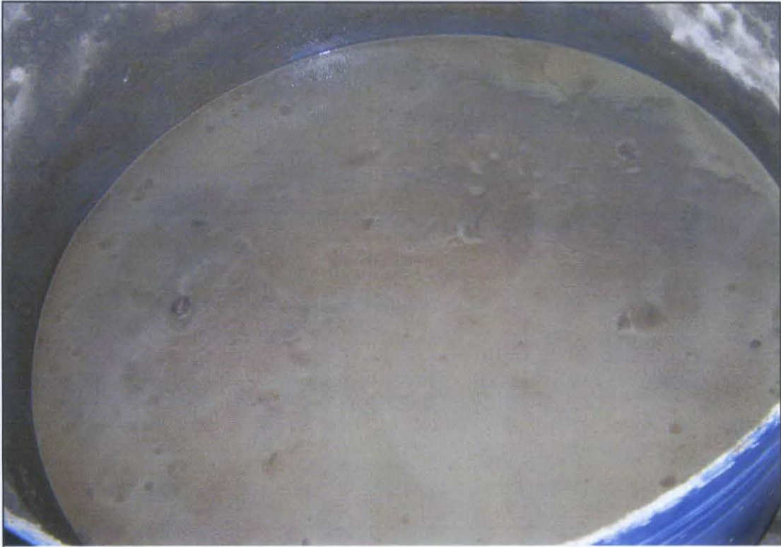
Figure B.1 High segregation occurred in mixture of size range 14 mm - 20 mm
