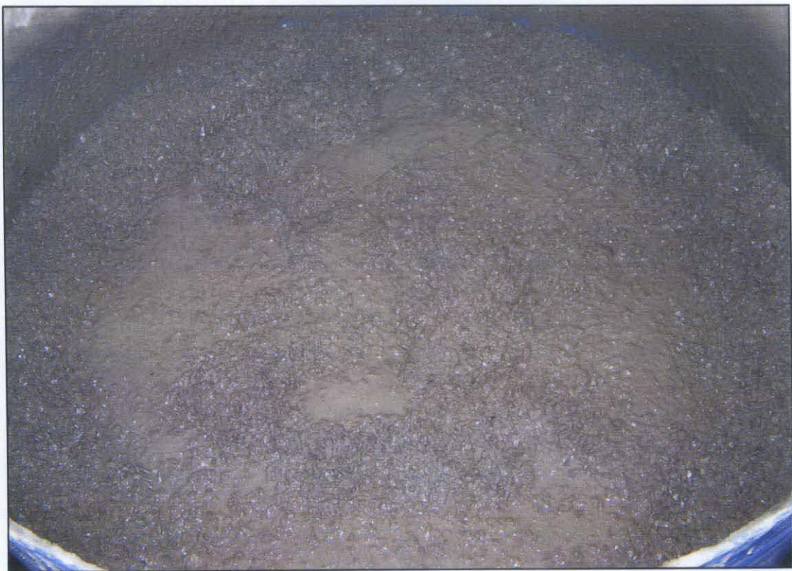
Figure B.4 Low segregation occurred in mixture of size range 3.36 mm – 20 mm
