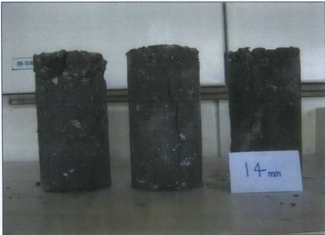
Figure F.2 After compressive strength test of size range 14 mm - 20 mm
