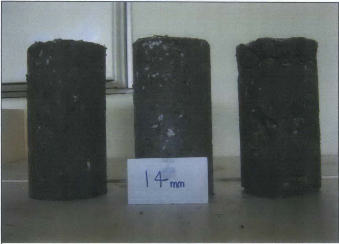
Figure F.1 Before compressive strength test of size range 14 mm - 20 mm
