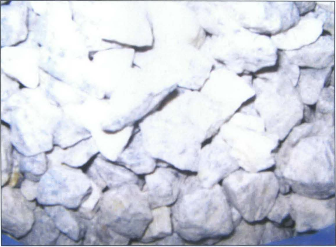
Figure I.1 Coarse aggregate of size range 14 mm - 20 mm
