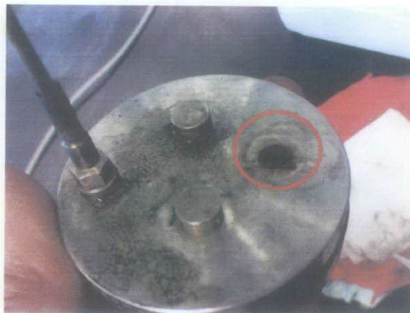
Figure A-6: Failure Part That Cause Explosion
