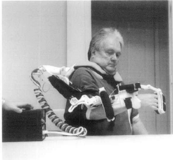
Figure 4: A robotic device used by stroke patients to retrain their muscles.
