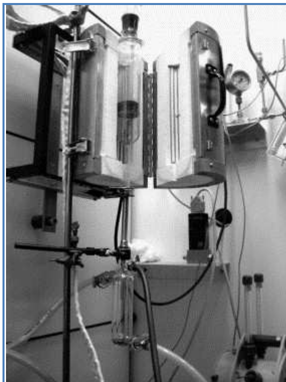
Figure 2.5: Bench-scale experimental set-up for wood torrefaction.
