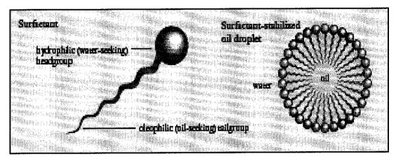
Figure 2.3 Surfactants consist of two parts; the water-seeking hydrophilic head group and an oil-seeking oleophilic tail group. This allows them to stabilize oil droplets.[5]
