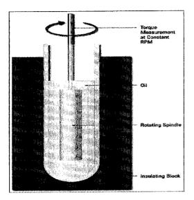
Figure 4.2 Rotary Viscometer
