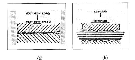
Figure 2.1 Lubrication system (a) Boundary Lubrication (b) Hydrodynamic Lubrication
