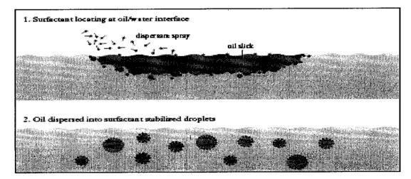
Figure 2.4 Surfactant locating at oil/water interface, and oil dispersed into surfactantstabilized droplets.[5]
