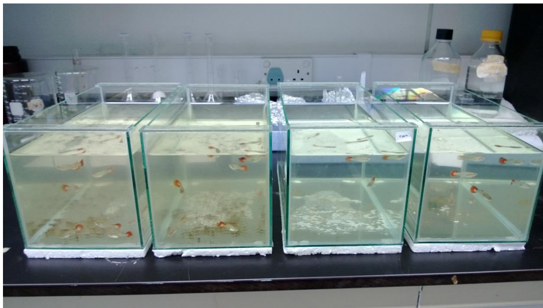
Figure 3.5: An initial test of influent WTP Teluk Kepayang with two replicates and a control tank
