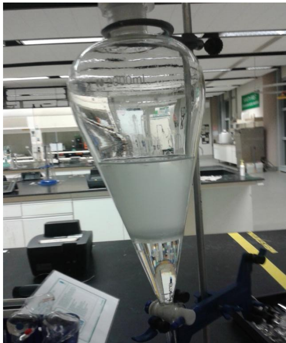
Figure A.5.2: The liquid- liquid extraction of the sample by using filter funnel
