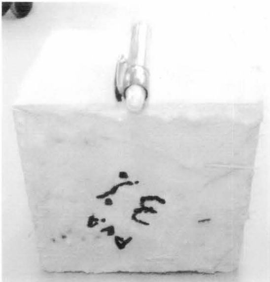
Figure 6h and 6i Pictures show the crack at the side of concrete samples with 3% fiber content
