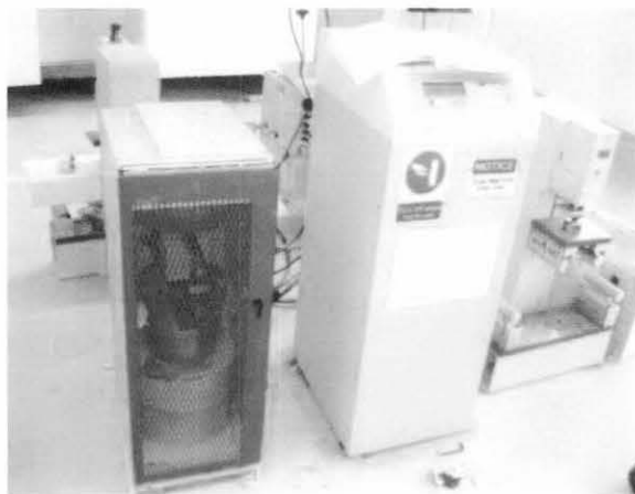
Figure 6g Compression which is used to test on concrete with fiber content 2% and 3%
