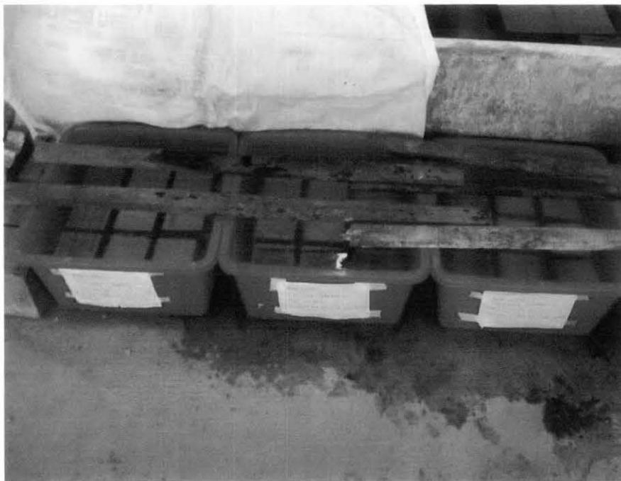
Figure 4a Curing tank for all samples. From left; curing tank of fiber content 1%, 2 and 3%
