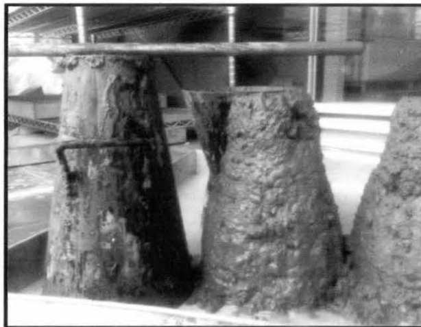
Figure 5.13 : Slump of concrete with 0% fiber
