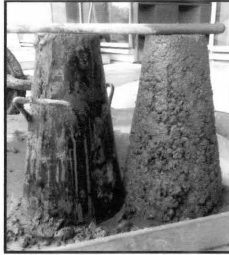
Figure 5.14 : Slump of concrete with 2% fiber
