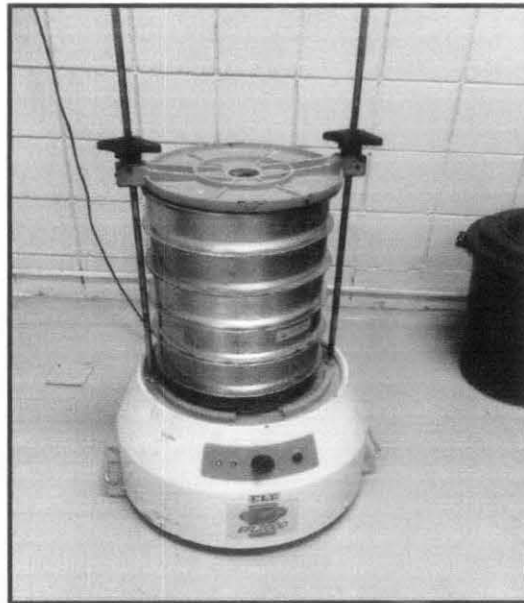
Stack of Sieve in a Mechanical Sieve Shaker
