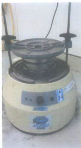
The blendered pineapple peel is sieved to get coarse size which is more than 212 micron
