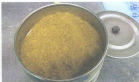
The blendered pineapple peel is sieved to get coarse size which is more than 212 micron
