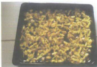
Pineapple peel waste cut into small pieces and dried further in oven for 16 hours at 80°
