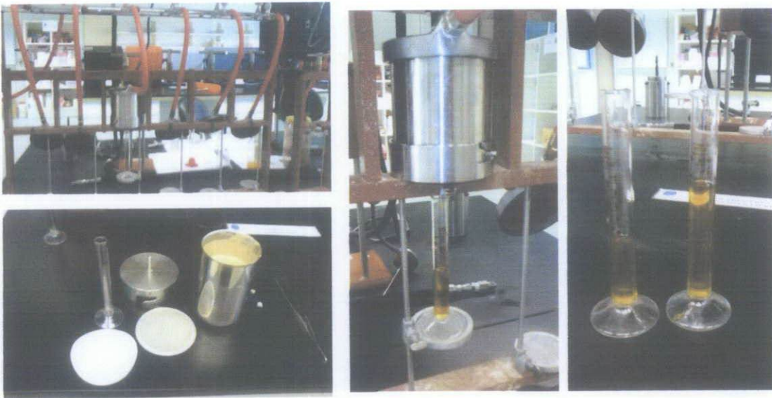
Mud filtration test using Low Pressure Low Temperature (LPLT) filter press
