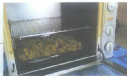
Pineapple peel waste cut into small pieces and dried further in oven for 16 hours at 80°
