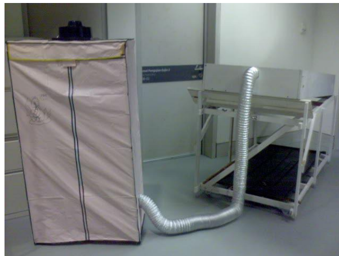
Figure 3.5: Actual prototype of the solar closet
