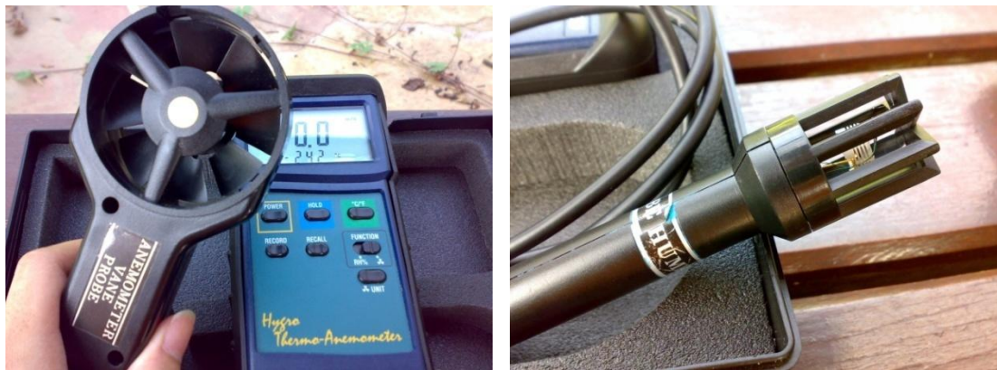
Figure 3.6: Hygro-Thermo-Anemometer with a) anemometer vane probe + temperature sensor b) humidity probe + temperature sensor
