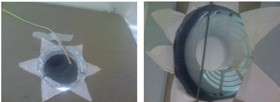
Figure 3.10: Thermocouple position at a) closet inlet b) closet outlet
