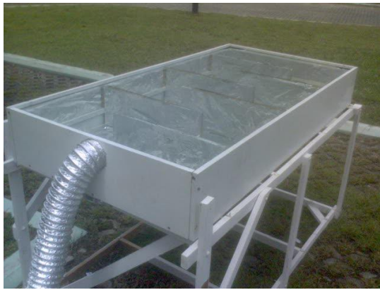
Figure 3.4: a) Air solar collector b) The plastic closet
