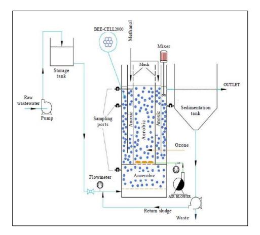
Figure 2: Schematic Diagram of the IFAS Pilot-Plant (Mehrdadi et. al., 2006)
