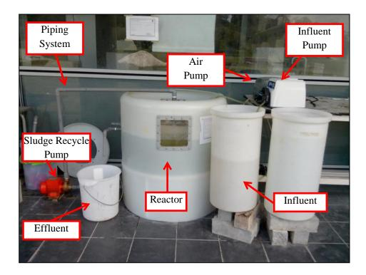
Figure 6: Setup Arrangement of the Reactor
