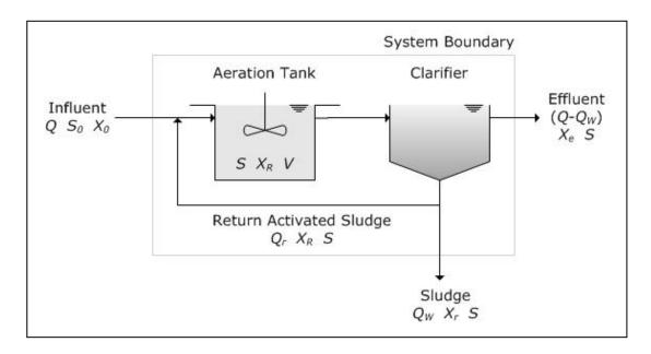
Figure 1: Activated Sludge Process Schematic Diagram (Lenntech B.V, 2008)
