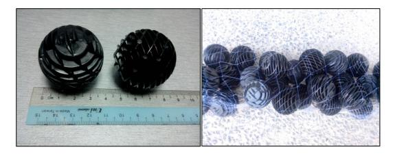
Figure 14: Configuration of the Bio-Balls
