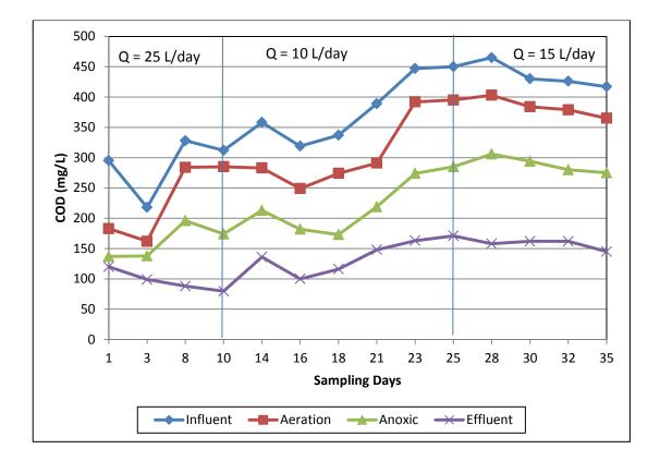
Figure 21: Graph of COD (mg/L) vs Sampling Days
