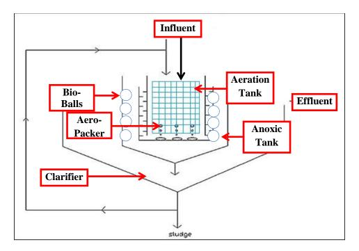
Figure 9: Schematic Diagram of the Reactor with Aero-Packer
