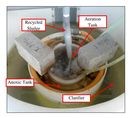
Figure 7: Top View of the Setup Arrangement of the Reactor
