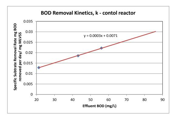
Figure 20: Graph of BOD Removal Kinetics, k.
