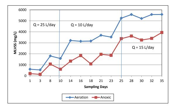
Figure 24: Graph of MLVSS vs Sampling Days
