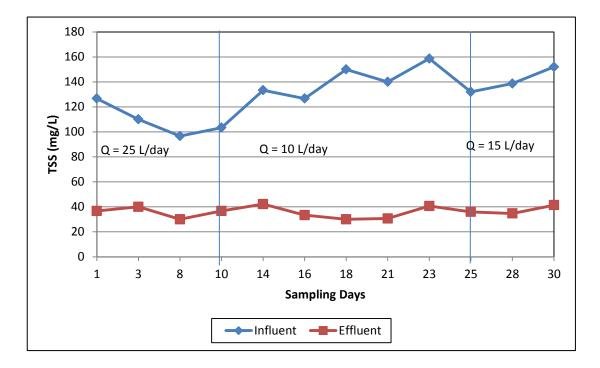
Figure 17: Graph of Total Suspended Solid (mg/L) vs Sampling Days
