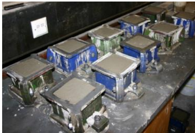
Figure 3.5 : Cast concrete in the 50x50x50mm cube
