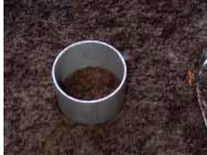
Figure 4.6: Fill the steel casing with WLP
