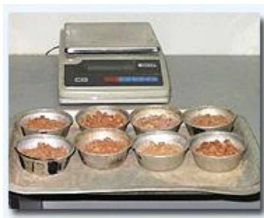
Figure 4.9: WLP after drying process
