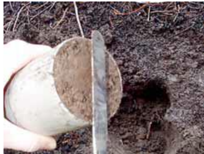
Figure 4.7: Level the steel casing with plate
