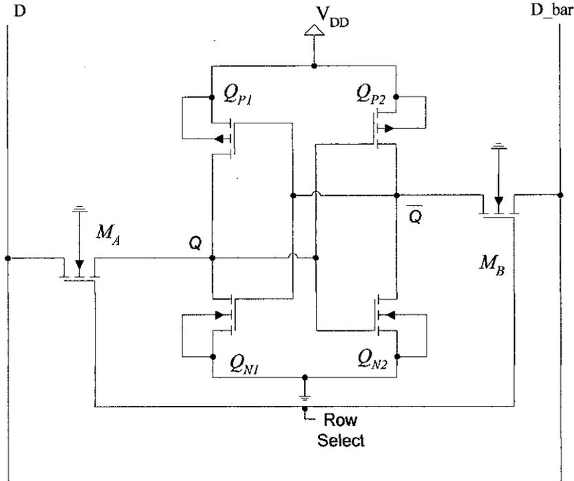
Figure 2 : 6T Cell Basic Memory Topology [11]
