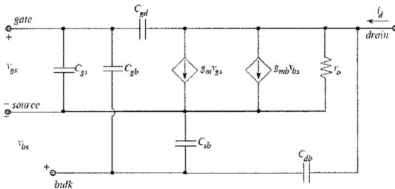
Figure 15 : MOSFET Small Signal Model [14]
