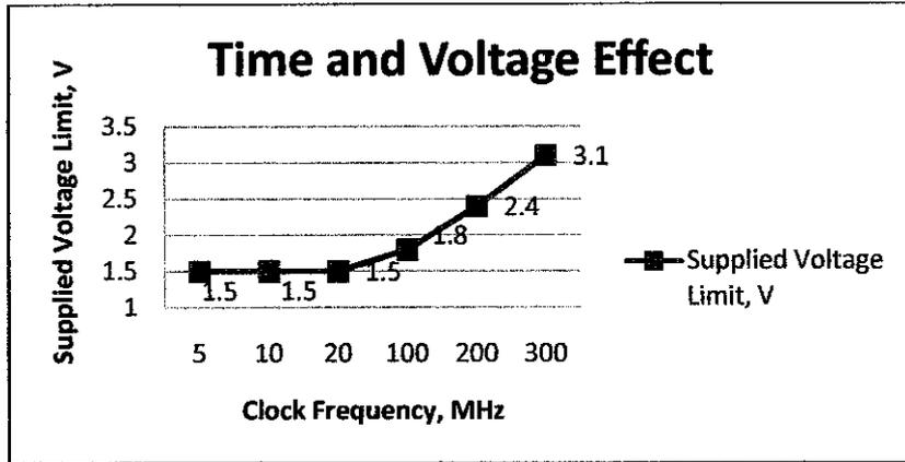
Figure 14 : Simulation Using ami16 Process Technology for Clock Frequency and Voltage Supply Effect
