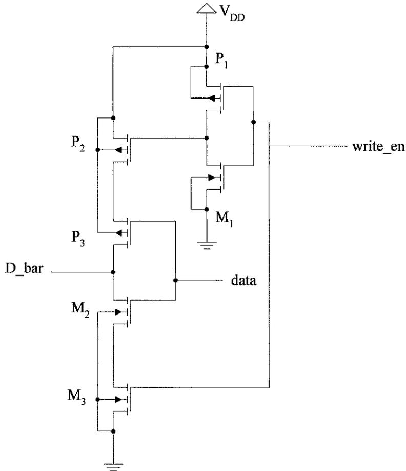
Figure 5 : Write Circuit for Input  $D_{\text{bar}}$
