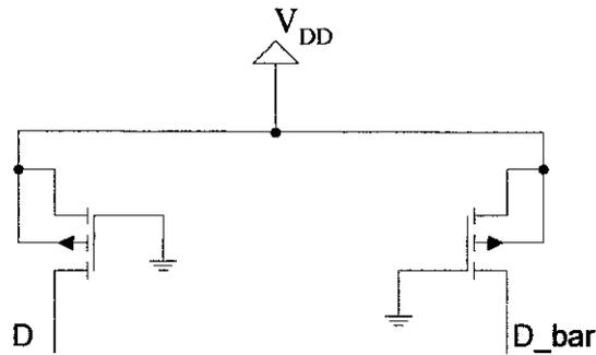
Figure 3 : Pull-up Circuit [5]
