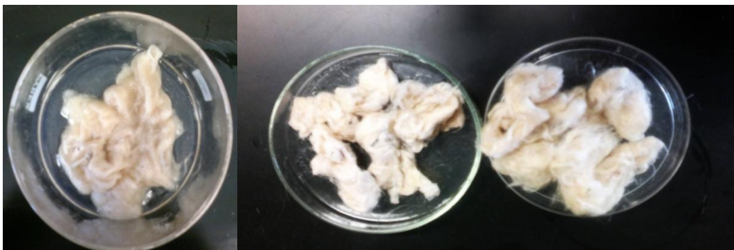
Figure 18: Image of (a) saturated kapok (b) wet kapok after the recovery process and (c) dry kapok ready for reusability
