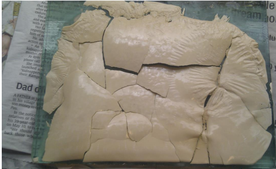
FIGURE 4-7: Sample 13 - Cracked Membrane (BPDA-ODA/DMAc)
