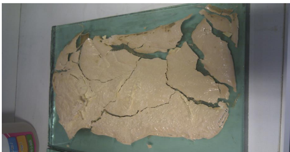
FIGURE 4-4: Sample 8 – Less-cracked Membrane (BTDA-ODA/DMF)
