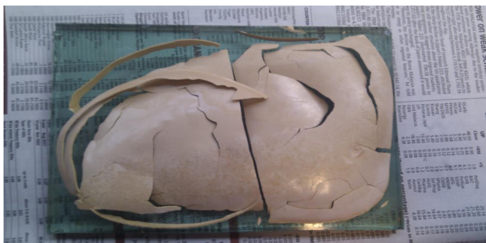
FIGURE 4-5: Sample 10 – Less-cracked Membrane (BTDA-ODA/DMAc)
