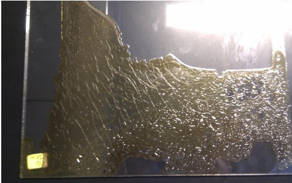
FIGURE 4-2: Sample 2– Cracked and Brittle Film without binder (BTDA-ODA/DMAc)
