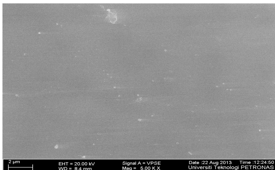
FIGURE 4-11: Surface View of BPDA-ODA Membrane
