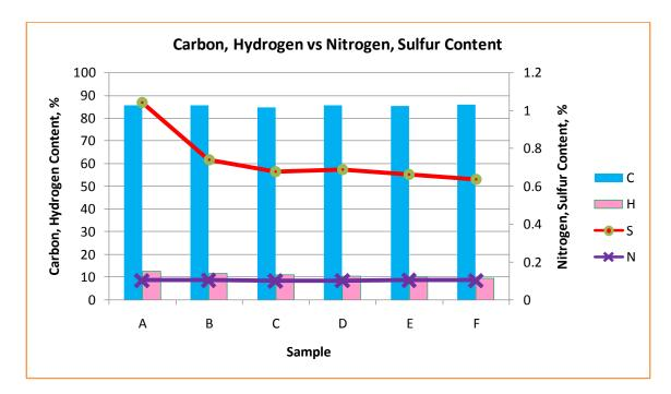
Figure 27: Carbon, Hydrogen, Nitrogen and Sulfur Content for different samples
