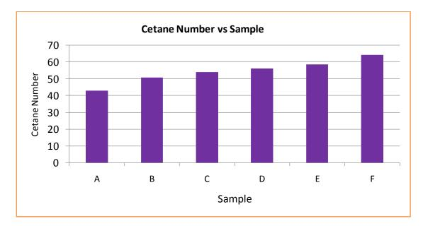
Figure 29: Value of cetane number for different samples
