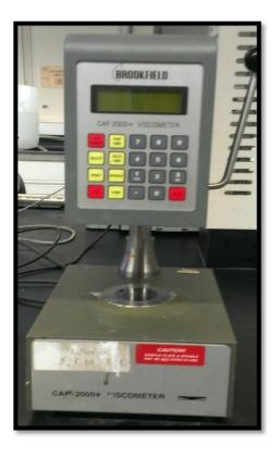
Figure 8 : Viscometer to measure viscosity
