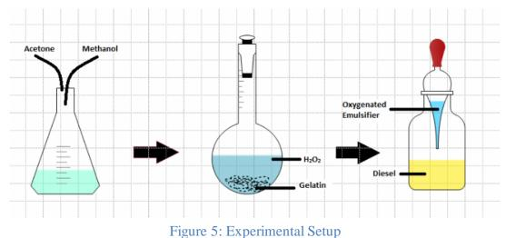
2. Stability test of hydrogen peroxide/diesel blend.
