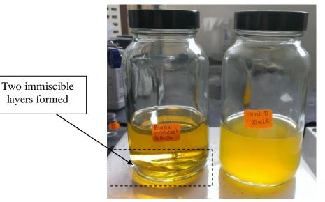
Figure 14 : Different between crude oil with hydrogen peroxide (left) and emulsified crude oil (right)
