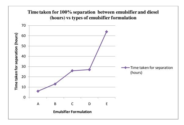
Figure 12 : Time taken for 100% separation between emulsifier and diesel (hours) vs types of emulsifier formulation
