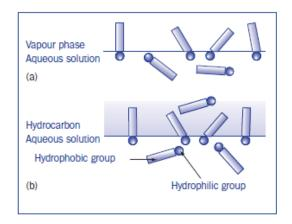
Figure 4 : Orientation of amphiphiles (a) solution– vapours interface and (b) hydrocarbon–solution interface <sup>[21]</sup>
