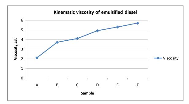
Figure 26: Kinematic viscosity value for different emulsified diesel sample
