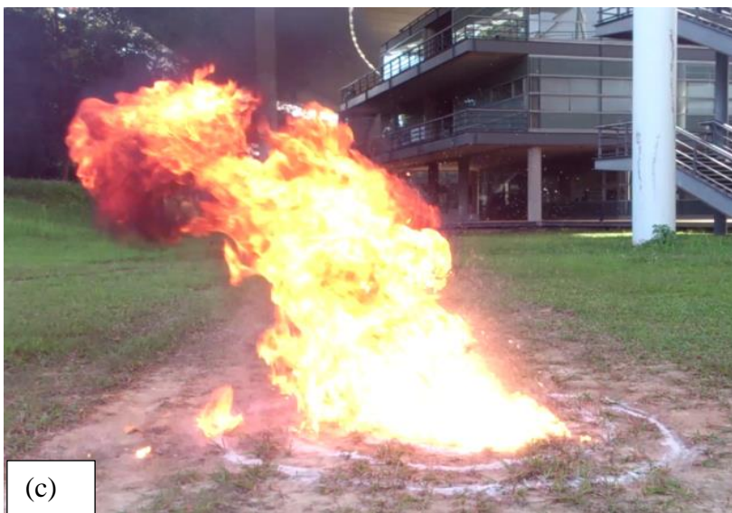
Figure 11: The boilover at different fuel composition. (a)70% Diesel-30% Petrol, (b) 60% Diesel-40% Petrol and (c) 50% Diesel-50% Petrol
