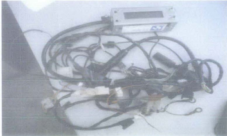
Figure 11: The wiring use with the throttle body injector (TBI)
