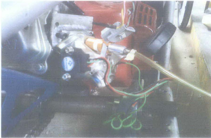
Figure 19: the vertical position of injector at the intake manifold
