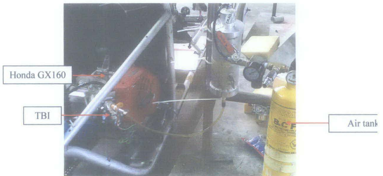
Figure 14: Setup for the experiment with TBI system
