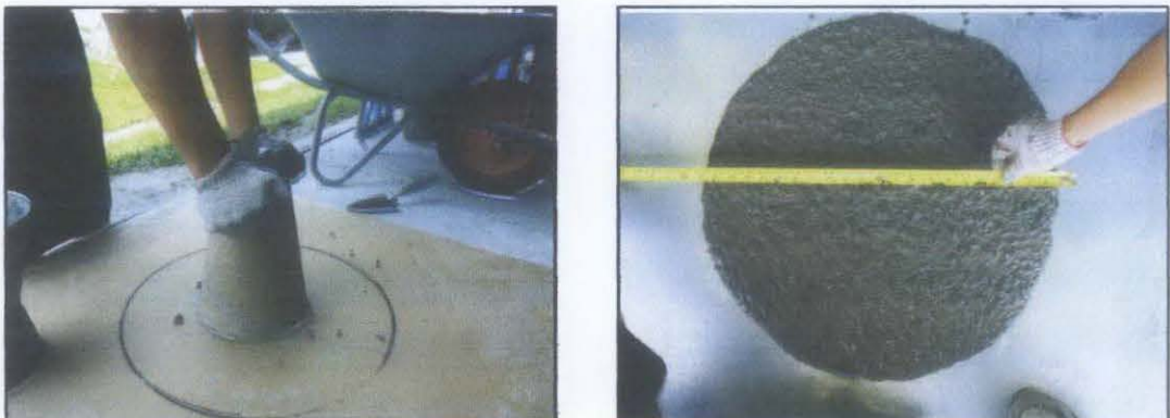
Figure 2: Slump Flow Measurement
