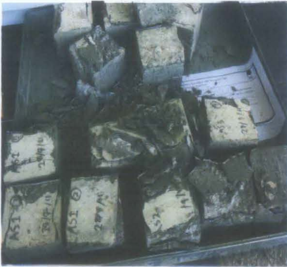
Concrete cube after testing
