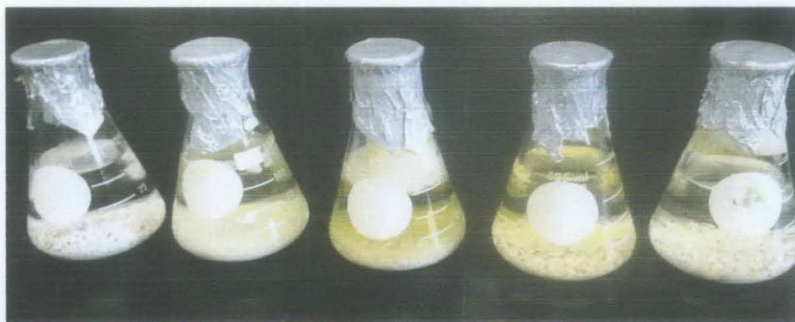
Figure 13: Sample after being heated 24 hours. From the left: without scale inhibitor, PASP 1000ppm, PASP 5000ppm, DTPMPA 5000ppm, DTPMPA 1000ppm all at pH 7 and 90°C
