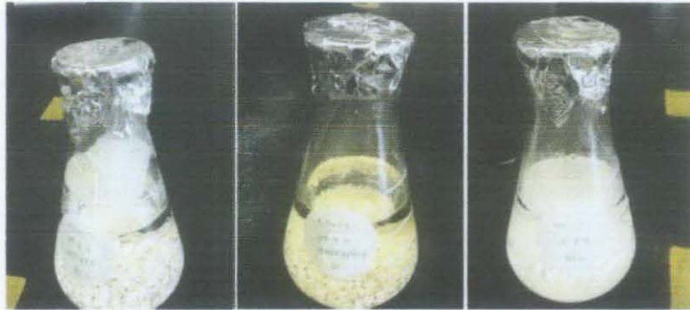
Figure 17: Sample after being heated for 24 hours. From left: DTPMPA 1000ppm, DTPMPA 5000ppm and without scale inhibitors all at pH 8.6, 50°C
