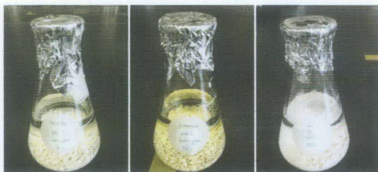
Figure 15: Sample after being heated for 24 hours. From left: DTPMPA 1000ppm, DTPMPA 5000ppm and without scale inhibitors all at pH 7, 50°C
