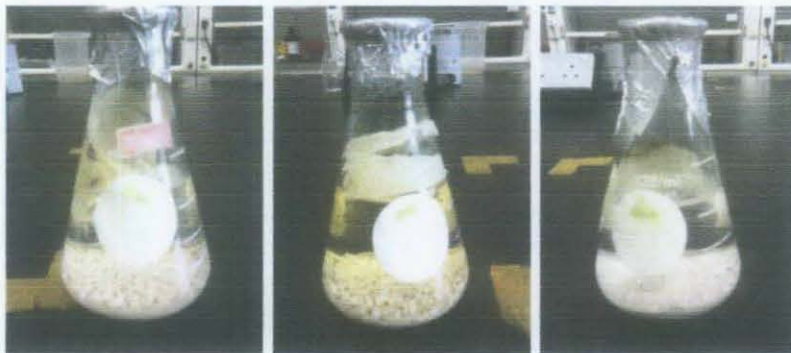
Figure 19: Sample after being heated for 24 hours. From left: DTPMPA 1000ppm, DTPMPA 5000ppm and without scale inhibitors all at pH 8.6, 90°C
