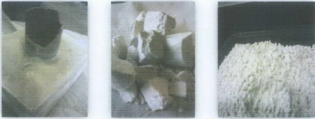
Figure 10: From left: the limestone from formation, limestone been crushed to smaller cube, smaller size of crushed limestone
