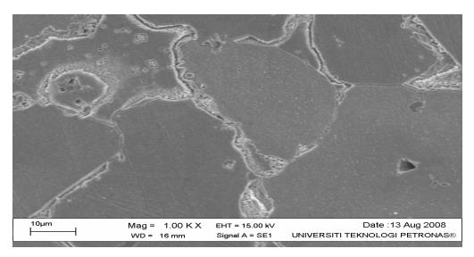
Figure 4.2: SEM photograph of failed propeller (100X)
