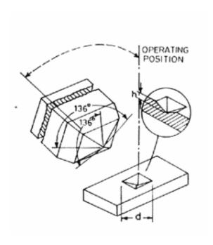
Figure 3.7: Vickers hardness test principle [15]
