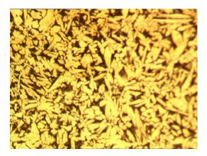
Figure 4.4(a) Micrograph image for new developed propeller material (100X)
