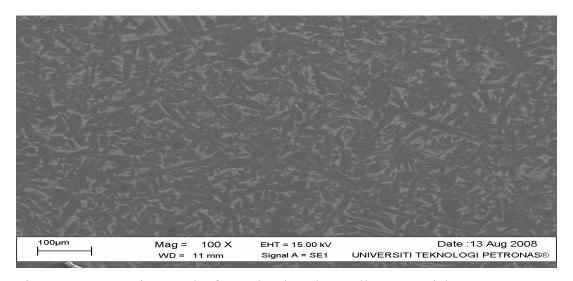
Figure 4.5: SEM micrograph of new developed propeller's material
