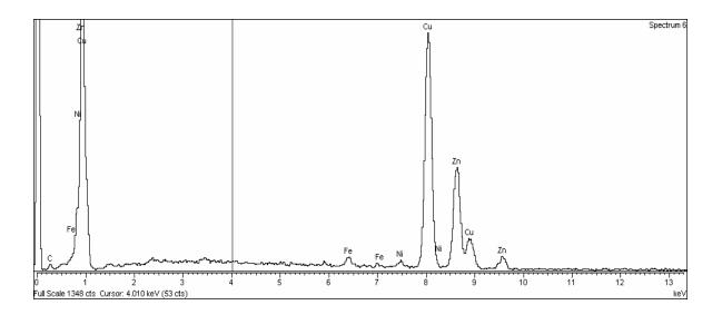
Figure 4.6: Qualitative analysis showing the elements present in failed propeller
