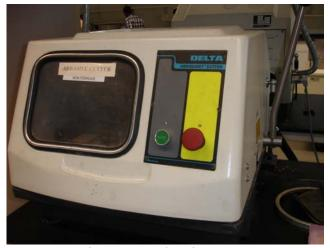
Figure 3.1: Abrasive cutter
