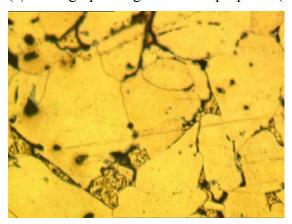
(b) Micrograph image of failed propeller (200X)
