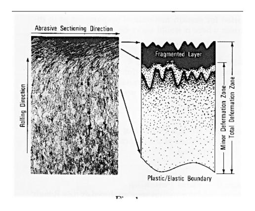
Figure 3.2: Rolling and Abrasive Sectioning Direction[9]
