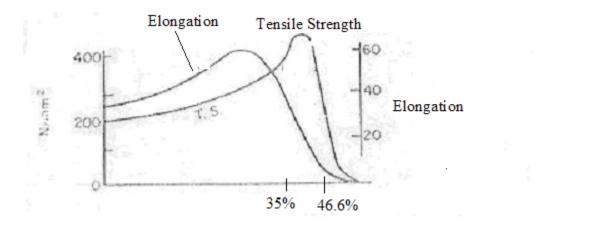
Figure 4.8(b): mechanical properties of brass [10]
