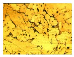
(a) Micrograph image for failed propeller (100X)
