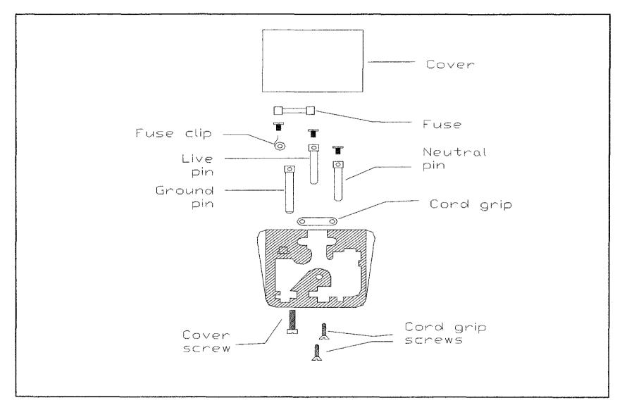
Figure 4.1: CAD drawing for three pin power plug subassembly
