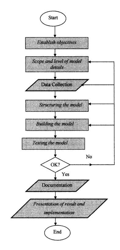
Figures 3.1: Modeling flow chart using WITNESS simulation [2]
