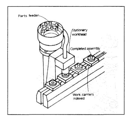
Figure 4.10: In-line indexing machine [1]
