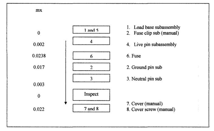
Figure 4.9: Station layout of in-line indexing machine [1]
