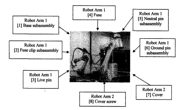
Figure 4.4: Single station Two-arm robot assembly for 3 pin power plugs
