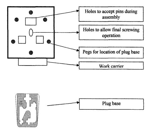
Figure 4.8: Work carriers suitable for holding and transferring three pin power plugs
