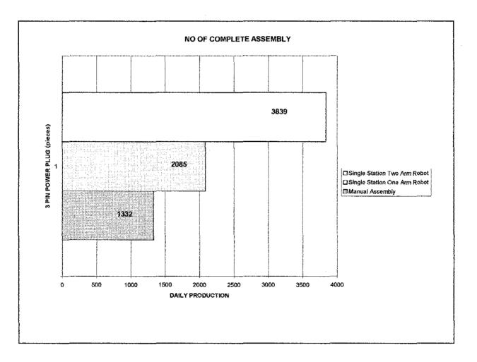
Figure 5.10: Comparison for daily production of 3 pin power plug
