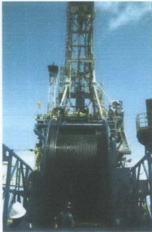
Figure 3: The coiled tubing unit (The treatment fluid are pumped through the coiled tubing to exit open-ended, a wash nozzle or a rotating jetting head)
