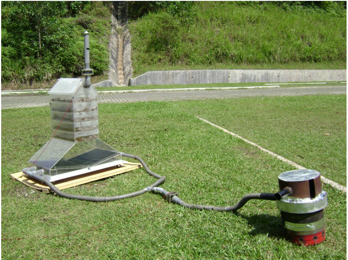
Figure 6.0: Complete connection of hybrid solar dryer with biomass integration (experimental setup)
