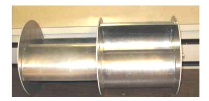
Figure 2.10: Double stage Savonius rotor
