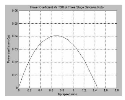
Figure 2.13: Graph of power coefficient versus tip speed ratio of a Three Stage Savonius rotor
