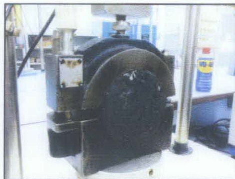
Figure 12 Marshall Stability Test
