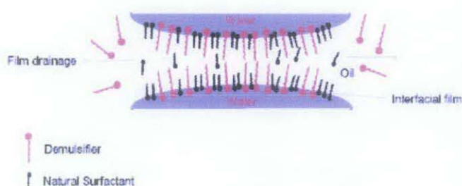
Figure 2.5: Film drainage in the presence of demulsifiers which displace the natural surfactants
