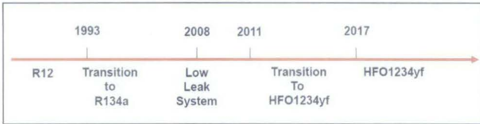
Figure 2.2: The phase out of refrigerant with GWP > 150[14]
