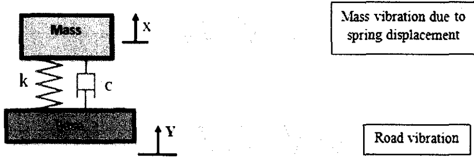
Figure 6: Simplified prototype spring-mass-damper model [17]
