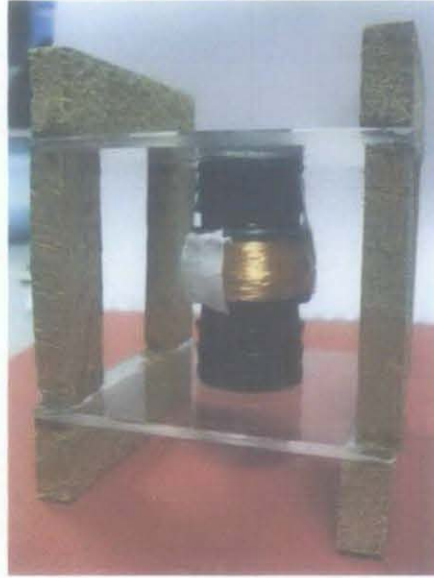
Figure 19: Stator and winding attached to the perspex sheet
