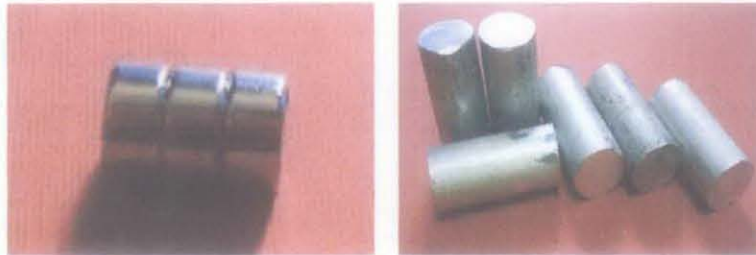
Figure 15: Magnets and aluminium rod for the rotor
