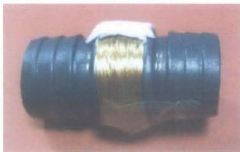
Figure 17: Stator and winding
