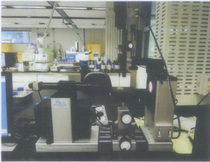
Figure 3.11: Optical Contact Angle Measuring Device: OCAH 200
