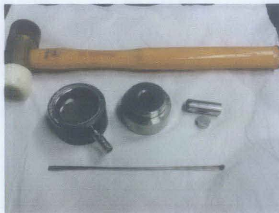
Figure 3.7: Apparatus used to fill in powder into metal casing
