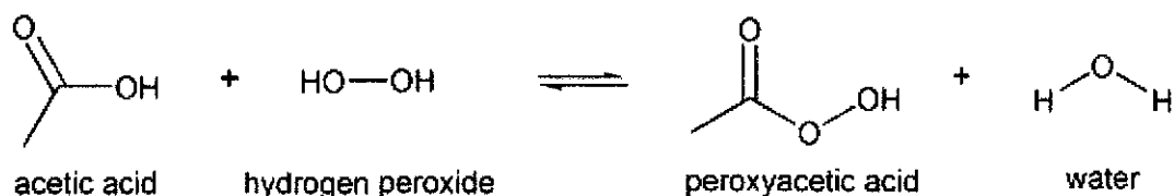
Figure 2.1: reaction of acetic acid and hydrogen peroxide
